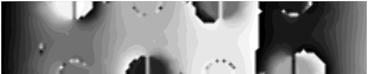
FIG. 7: The phase of the electric field component E_y at 10.064 GHz for a structure as in Figs. 6(a), 6(b) with four layers of spheres. The feeding plane is on the left, and the energy propagates from left to right. The black color corresponds to -\pi and the white to +\pi . The phase is increasing as the distance from the source increases, which indicates that the wave is a backward wave.
