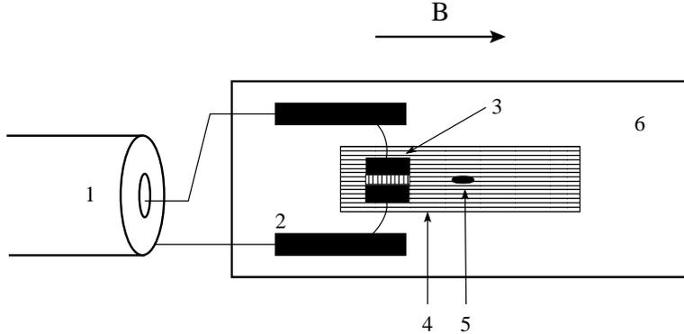
FIG. 2: Experimental set-up. The microwave signal is taken by a coaxial cable (1) through a pair of conducting stripes (2) to the transducers (3), which generate the surface acoustic waves on the  $\text{LiNbO}_3$  substrate (4). The  $\text{Mn}_{12}$  crystal (5) is glued directly on the substrate, with the easy anisotropy axis parallel to the magnetic field direction. The whole assembly is mounted on a plastic stand (6).
