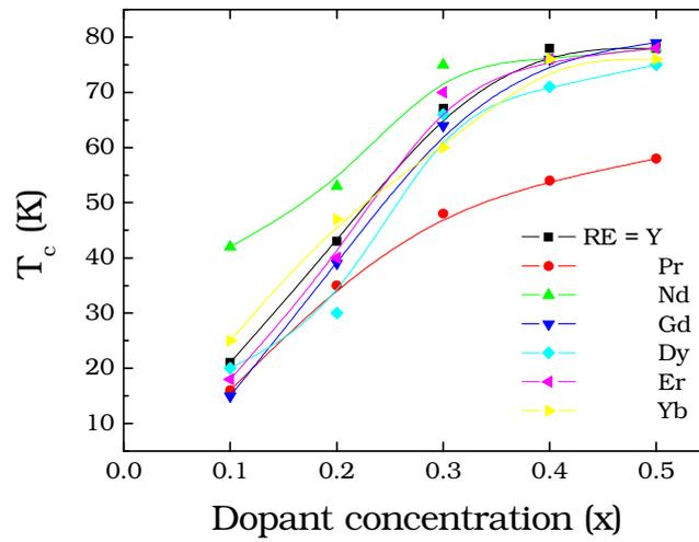
**Fig. 8**  $T_c$  vs.  $x$  for  $La_{2-x}RE_xCa_2xBa_2Cu_{4+2x}O_z$ .
