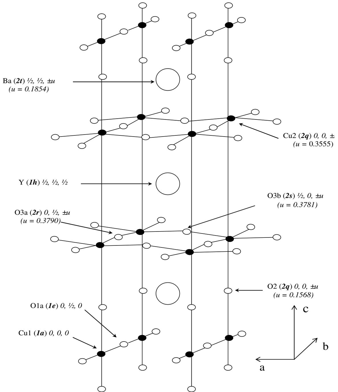
**Fig. 2** Structure of the orthorhombic unit cell of  $\text{YBa}_2\text{Cu}_3\text{O}_{7-6}$  ( $Pmmm$ ). Wyckoff notations and atomic positions are shown in parenthesis.
