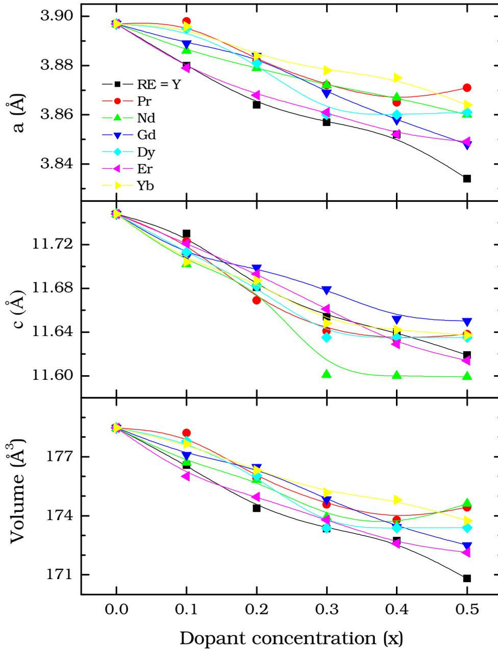
**Fig. 6** Decrease in the lattice parameters (*a*, *c* and *Volume*) with increasing dopant concentration for different RE substituted La-2125 compounds.
