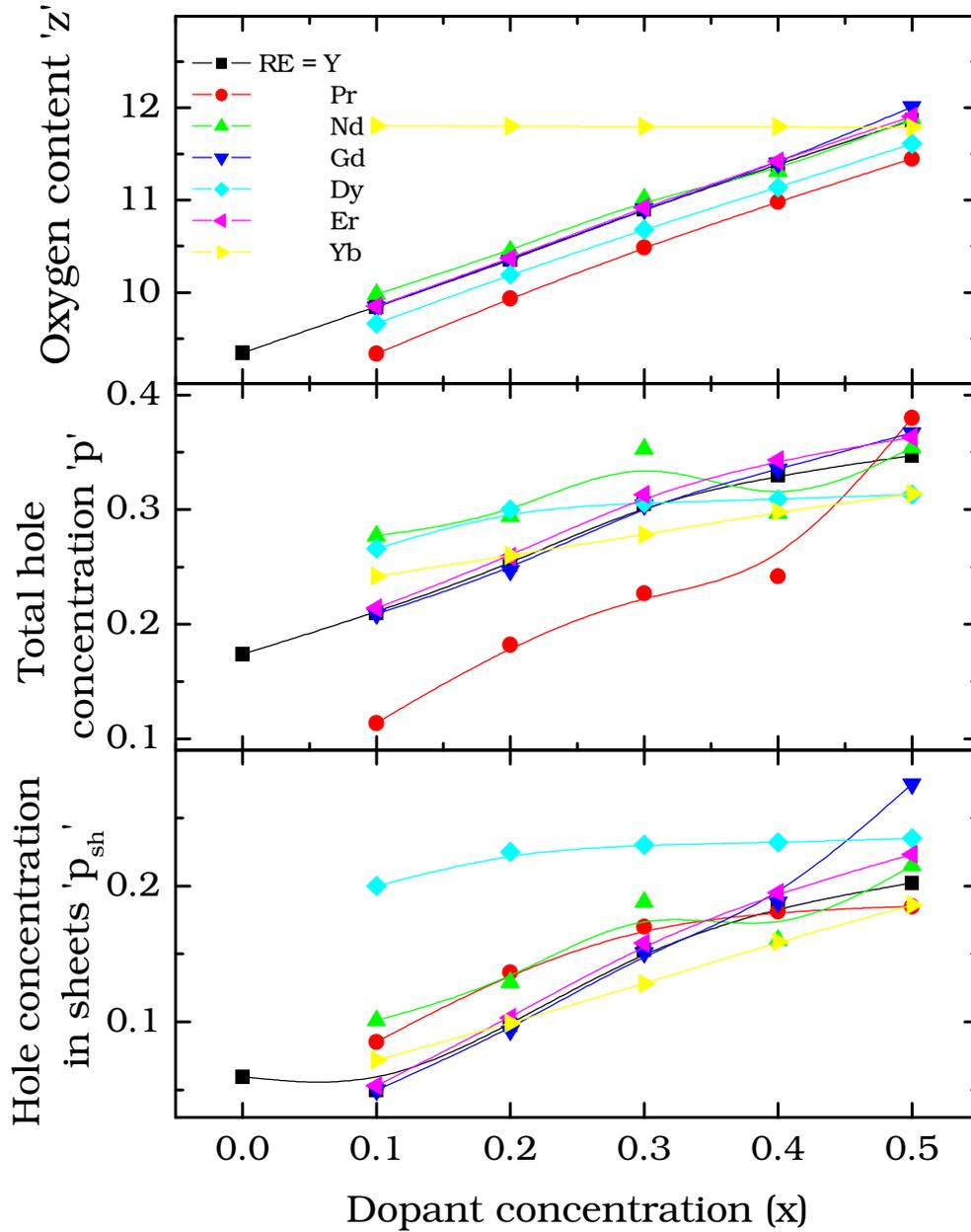
**Fig. 10** Oxygen content per formula unit obtained from Iodometric double titration experiment. Hole concentration has been calculated from oxygen content values.
