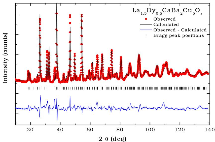
**Fig. 4 Neutron diffraction pattern for  $\text{La}_{1.5}\text{Dy}_{0.5}\text{CaBa}_2\text{Cu}_5\text{O}_z$  recorded at room temperature and fitted to a tetragonal triple perovskite unit cell (La-123 type) using Rietveld method.**
