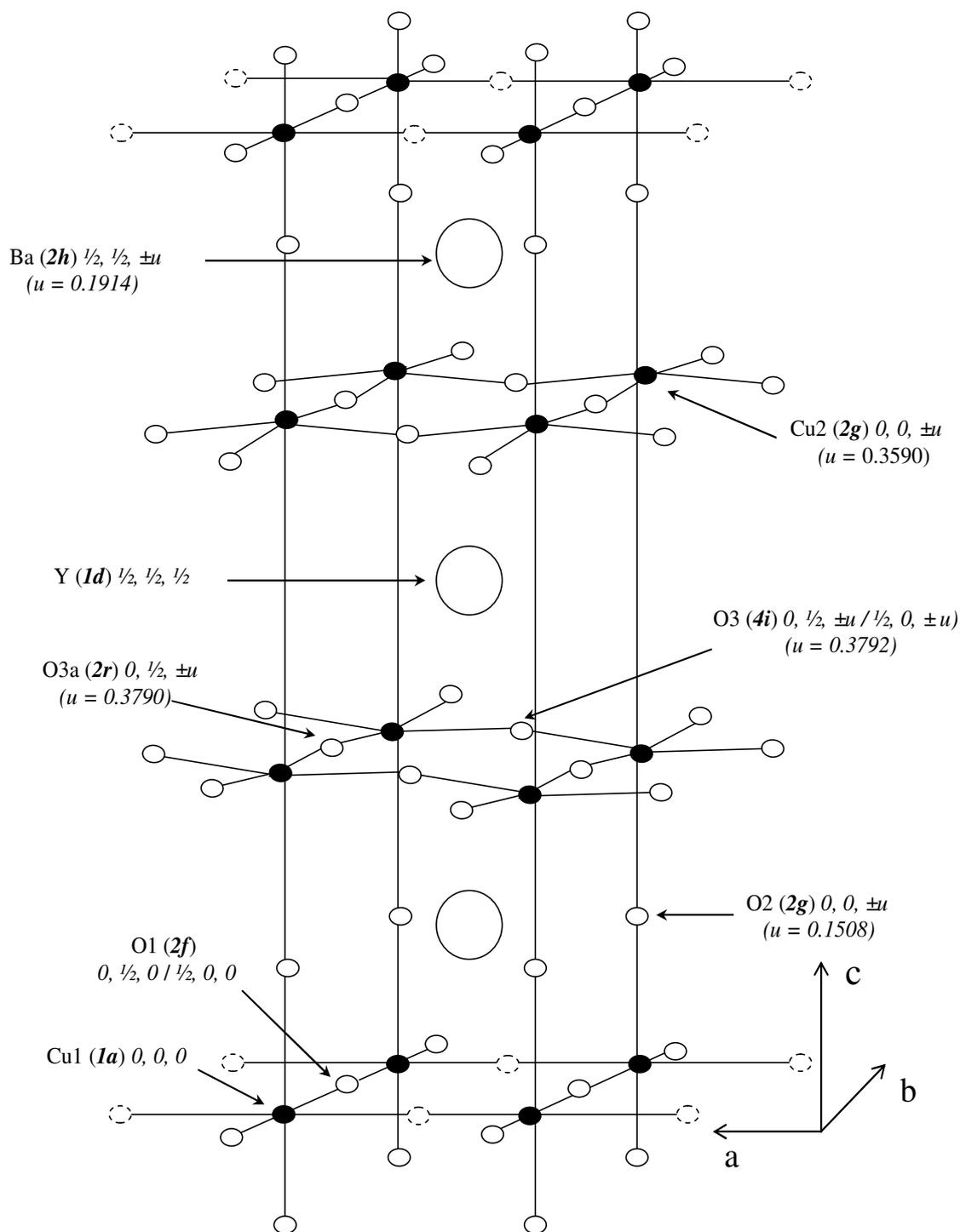
**Fig. 3** Structure of tetragonal unit cell of  $YBa_2Cu_3O_6$  ( $P4/mmm$ ). Wyckoff notations and atomic positions are shown in parenthesis.
