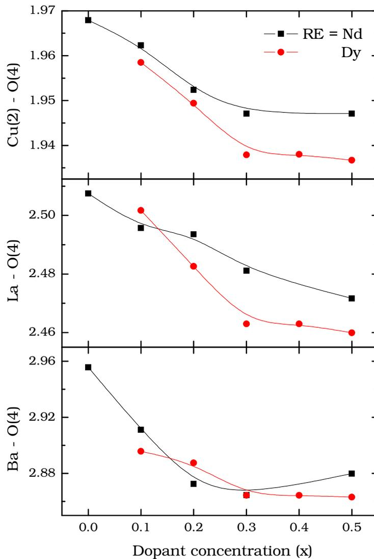
**Fig. 7** Variation in selected bond lengths with increasing dopant concentration.
