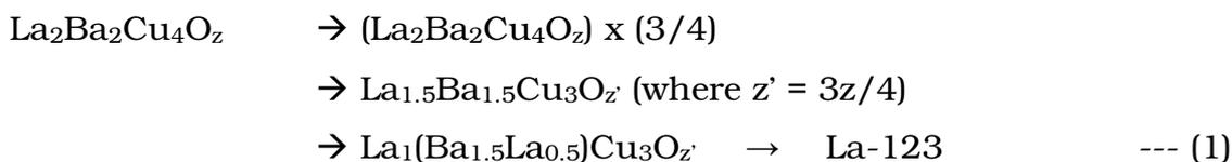
The Rietveld analysis of the powder neutron diffraction data of La-224 compound has confirmed the stoichiometric composition as shown in equation (1) and a structure similar to a tetragonal La-123 structure [16]. Similarly, the La-2125 compound can also be shown in La-123 composition as:
