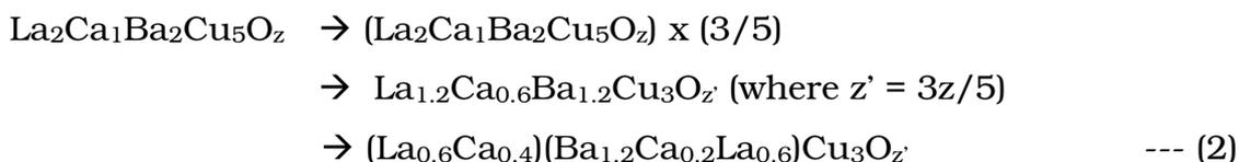
When  $\text{RE}^{3+}$  (where RE is rare earth, such as Dy, Nd, Pr, Gd, Er, Y etc) is substituted at  $\text{La}^{3+}$  site, then, for  $x = 0.5$ , the La-2125 compound with  $\text{RE}^{3+}$  can be represented as:
