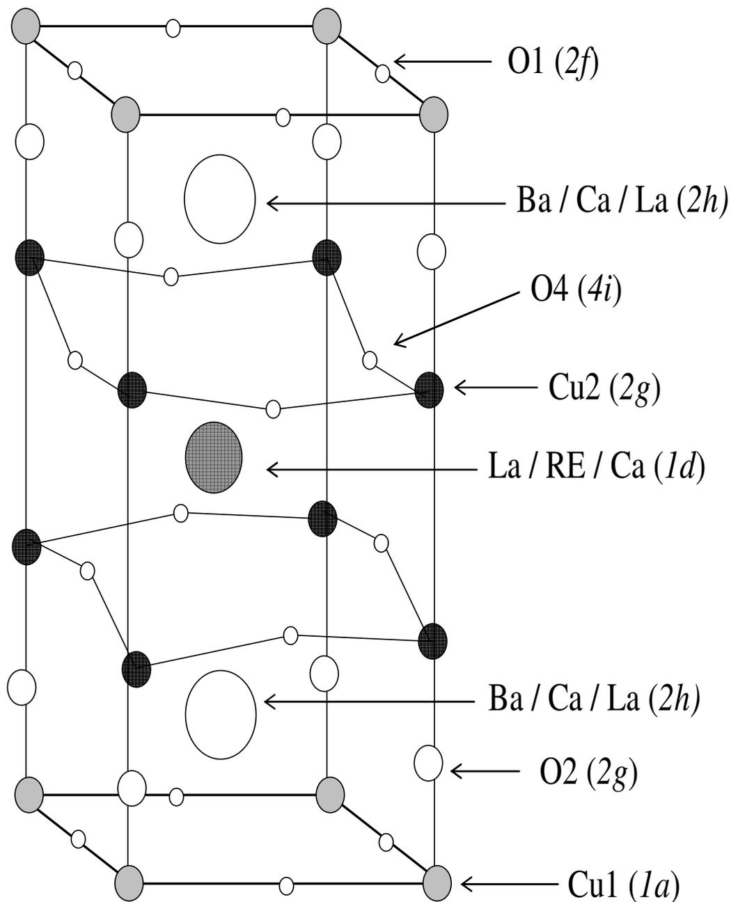
**Fig. 5** The structure of the La-2125 unit cell, derived from the tetragonal La-123 structure. Wyckoff positions are represented in parenthesis.
