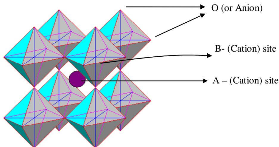
**Fig. 1 Simple cubic perovskite structure**
