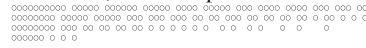
FIG. 11: Winding pattern cross section for 87 Rb Zeeman slower consisting of three solenoids. Each drawing represents half of the cross section of each a solenoid. The “O”s represent wires, while the spaces between the wires were meant to be smoothed out to an average value during construction. Each character in the drawing represents a physical size of 3.5 mm. The wire is hollow core water cooled copper, identical to that used in construction of the magnetic trap as described in C3. The high current coil is closest to the main chamber. The single layer uniform bias coil is not depicted.
