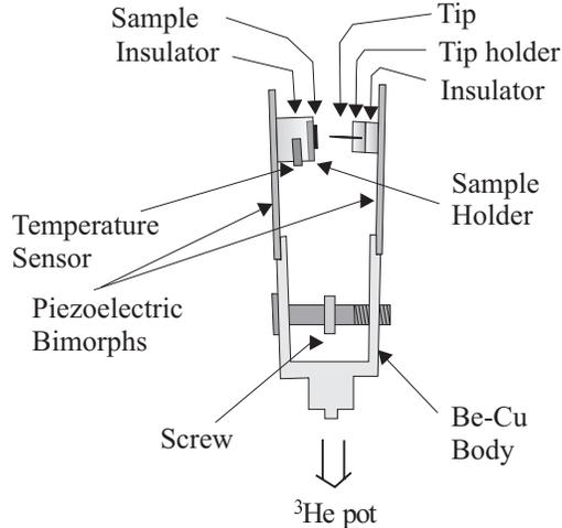
**Figure 1.** A schematic drawing of the point-contact spectroscopy rig (not to scale). A point contact is formed by bringing a tip and a sample into contact using a fine screw. It is kept stable by adjusting the  $dc$  voltage to the piezoelectric bimorphs while being cooled down. The main body is made of Be-Cu to ensure a reversible movement when adjusted by the screw.
