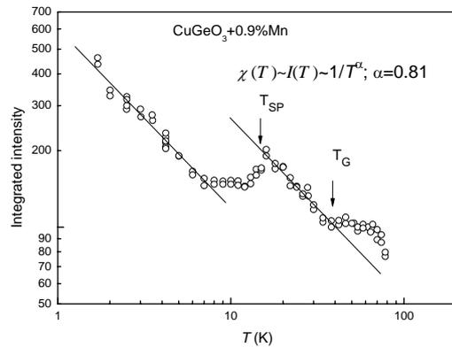
Fig. 2. Temperature dependence of the integrated intensity for 210 GHz. Solid lines represent power asymptotic of magnetic susceptibility (Eq. (1)). Arrows mark transitions into Griffiths ( $T_G$ ) and spin-Peierls state ( $T_{SP}$ ).
