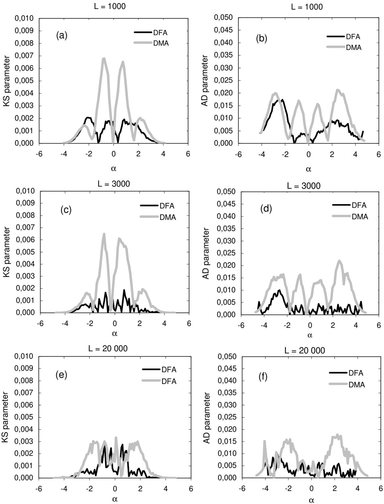
Figure 10: Kolmogorov-Smirnov (a) (c) (e) and Anderson-Darling (b) (d) (f) tests of correspondence between obtained distributions and the Gaussian one drawn respectively for time series of length  $L = 1000$ ;  $L = 3000$ ;  $L = 20000$
