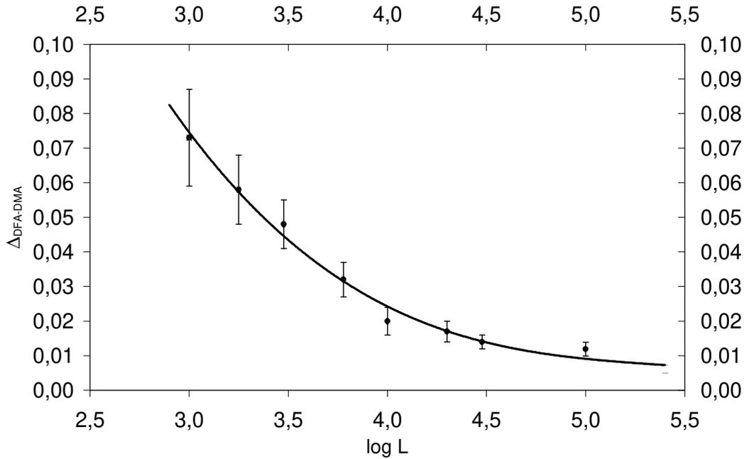
Figure 13: A mean difference  $\Delta_{DFA-DMA}$  between DFA and DMA exponents calculated for the same series as a function of the series length  $L$ . Marked error bars  $\Delta_{DFA-DMA} = \Delta_{DFA} + \Delta_{DMA}$  correspond to uncertainties in slope determination in regression analysis for both methods.
