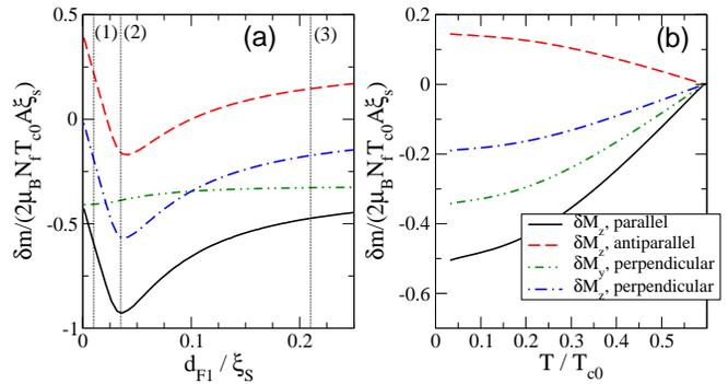
FIG. 4: (a) Change in magnetic moment  $\delta\vec{m}$  of a trilayer as function of the layer thickness  $d_{F1}$ , for  $d_S = 4\xi_S$ ,  $d_{F2} = 0.1\xi_S$ ,  $T = 0.1T_c$ , and  $J_1 = J_2 = 20T_c$ . The other parameters are as in Fig. 2. (b) The temperature dependence of  $\delta\vec{m}$  for parameters as in (a), but with  $d_{F1} = 0.2\xi_S$ . The vertical lines in (a) are referred to in Fig. 5.
