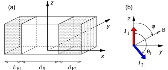
FIG. 1: The trilayer consists of a superconductor of thickness  $d_S$  and two ferromagnets of thicknesses  $d_{F1}$  and  $d_{F2}$ . The exchange fields of the ferromagnets,  $\vec{J}_1$  and  $\vec{J}_2$ , are confined to the  $y$ - $z$ -plane, but are misaligned by an angle  $\theta_J$ . For torque measurements, a small magnetic field is applied in the  $y$ - $z$ -plane at an angle  $\varphi$ .
