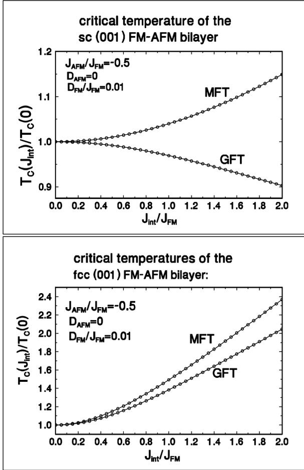
**Figure 4.** Critical temperatures  $T_C(J_{int})$  as a function of the interlayer coupling  $J_{int}$  of a simple cubic (upper panel) and a fcc (lower panel) FM-AFM bilayer ( $T_C$  is normalised to  $T_C(J_{int} = 0)$ ). Results with mean field theory (MFT) and with Green’s function theory (GFT) are compared. Note the qualitatively different behaviour of the GFT results for sc and fcc stacking (see the text).
