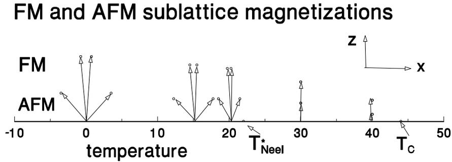
**Figure 3.** The reorientation of the sublattice magnetizations of the FM and AFM bilayer as a function of the temperature for the case of the strongest coupling ( $J_{\text{int}} = 160$ ) of figure 2.
