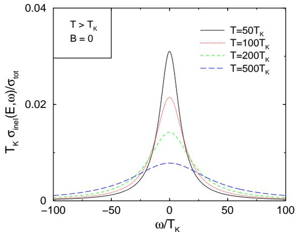
FIG. 1: (Color online) Differential cross-section,  $\sigma(E, \omega)$ , at large temperatures,  $T \gg T_K$ , without Zeeman splitting,  $B = 0$ , as given by Eq. (19). The Lorentz peaks have a width given by the Korringa relaxation rate  $1/\tau_K$ , Eq. (17).
