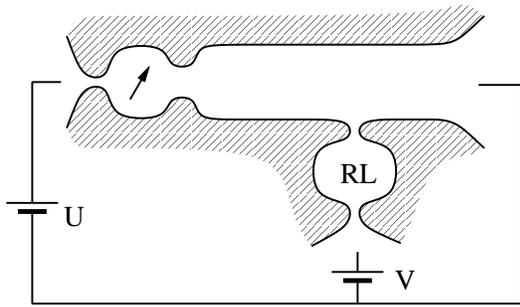
FIG. 7: Experimental quantum dot setup. A wire leads to a quantum dot in the Kondo regime (indicated by the arrow), which is in addition weakly connected to another reservoir at a voltage  $U$ . The resonance-level (RL) quantum dot acts as a probe.
