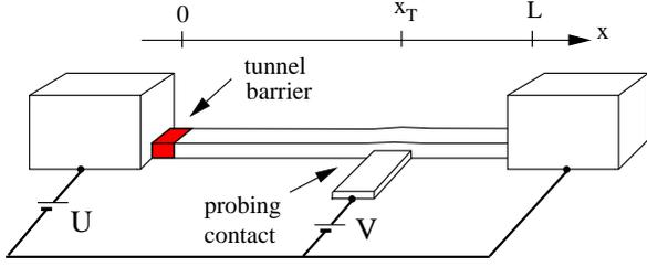
FIG. 6: (Color online) Experimental setup of Pothier *et al.*<sup>6</sup> with an additional tunnel barrier which limits the injection of hot electrons into the wire. The voltage drop across the wire is denoted by  $U$ . The voltage applied at the probing contact is  $V$ .
