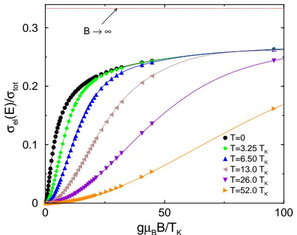
FIG. 3: (Color online) Weight of the elastic scattering cross-section,  $\sigma_{\text{el}}(E) = \int d\omega \sigma_{\text{el}}(E, \omega)$ , see Eq. (32), determined by NRG. The weight increases as  $B^2$  for small magnetic fields and saturates logarithmically slowly to the limiting value for large  $B$ , see Eq. (43).
