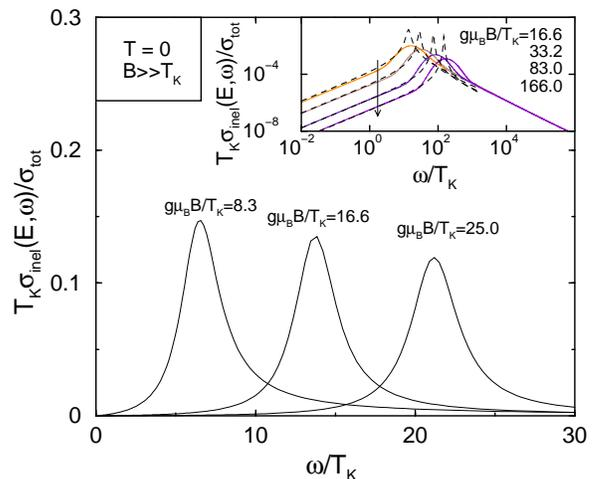
FIG. 5: (Color online) Inelastic scattering cross-section for several magnetic field values,  $B \gg T_K$ , at  $T = 0$  according to Eq. (44), which is applicable unless  $\omega \gg B$ . Note that the position of the resonance is shifted away from the Zeeman energy as described by Eq. (30). The inset shows the comparison of the analytical result (44) (dotted lines) with NRG calculation (colored lines). The low-frequency tail matches nicely. However, the NRG overestimates the width of the peak.
