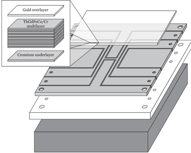
**Figure 4.** Schematic view of the hybrid atom chip. Inset: TbGdFeCo/Cr multilayer film and Au overlayer. From the top down, glass slide coated with magnetic film, machined silver foil H-wire and end wires, Shapal-M base-plate and Cu heat sink. Missing from the schematic is the second glass slide and two rubidium dispensers
