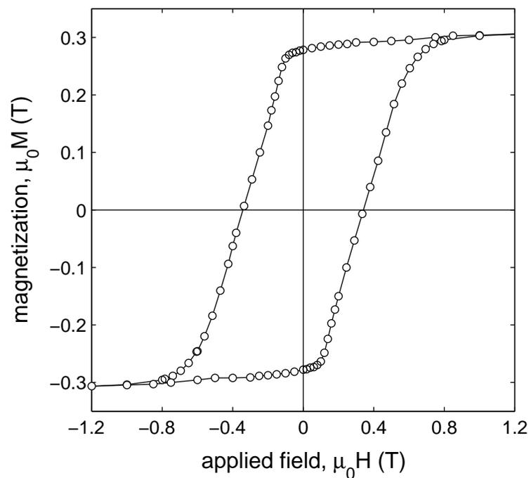
**Figure 2.** A hysteresis loop derived from SQUID magnetometry of a multilayer  $\text{Tb}_6\text{Gd}_{10}\text{Fe}_{80}\text{Co}_4$  magnetic film. The film magnetization is  $\mu_0 M_S \sim \mu_0 M_R = 0.28$  T and the coercivity is  $\mu_0 H_C = 0.32$  T.
