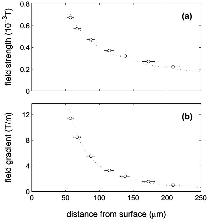
**Figure 6.** Measurements of the magnetic field strength (a) and field gradient (b) as a function of distance from the surface. The data (open circles) agrees well with predictions (dotted line) of the simple model (see Equation 1). Experimental errors are mostly determined by image resolution and a small uncertainty in the pixel size calibration.
