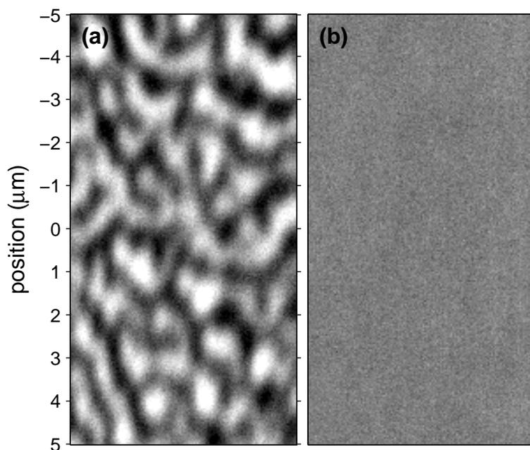
**Figure 3.** Magnetic Force Microscope (MFM) image of a  $\text{Tb}_6\text{Gd}_{10}\text{Fe}_{80}\text{Co}_4$  magnetic film surface. (a) Unmagnetized sample shows domain structure with micron sized features. (b) Uniformly magnetized sample is free of any visible magnetic structure.
