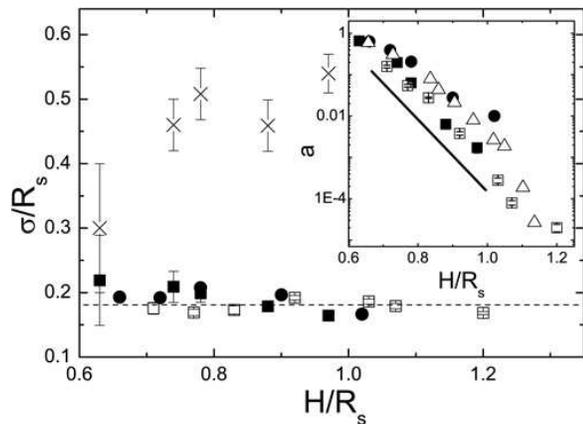
FIG. 5: Width of the shear profiles,  $\sigma$ , for different filling heights  $H$ . Data show  $\sigma$  both along the axial direction in the bulk (■ and □ from MRI experiments using different methods [13], ● from simulations) and along the radial direction in the surface layer (×). Dashed line is  $\sigma = 0.18R_s$ . Inset: offset  $a$  vs.  $H$  from MRI (■, □) and simulations (●). Surface data from Fig.1 are shown for comparison (△). Solid line indicates exponential behavior.
