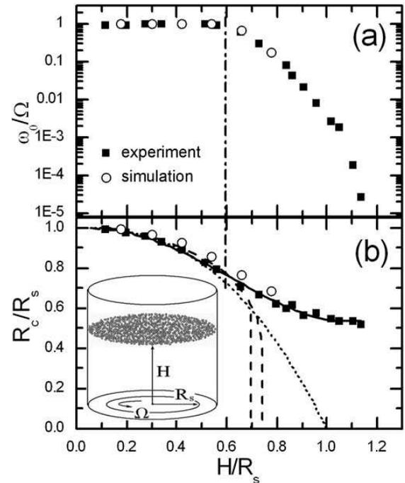
FIG. 1: Surface flow as function of filling height,  $H$ . (a) Angular velocity,  $\omega_0$  at the cell axis. (b) Center of the shear band,  $R_c$ . Solid line is a gaussian fit to guide the eye; dotted line is the fitting function of Fenistein *et al.* [7]; dashed line is the theoretical result [8]. Vertical dash-dot line indicates  $H = 0.6R_s$ . Inset: Schematic of split-bottom Couette cell.
