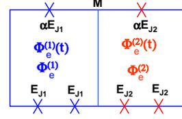
FIG. 1: (Color online) Two superconducting flux qubits are coupled through their mutual inductance  $M$ . Each qubit loop includes three junctions. The tunable interaction between two qubits can be realized by changing the frequency of the external magnetic flux  $\Phi_e^{(l)}(t)$  ( $l = 1, 2$ ) through the  $l$ th qubit.
