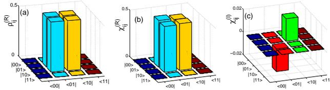
FIG. 2: (Color online) A schematic representation of tomographically measured state  $\rho$  [with only real part in (a)] for a completely decoupled system, as well as a state  $\chi$  [with real part in (b) and imaginary part in (c)] for a two-qubit system with large detuning—after considering a duration  $t$  before measuring the created state  $|\psi_+\rangle$ .
