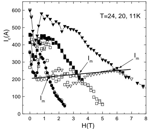
Figure 3: Field dependence of  $I_c$  for a carbon-nanotube doped  $MgB_2/Fe$  wire at  $T = 24, 20$  and  $11K$ , shown with round, square and triangle symbols, respectively. Open symbols are obtained with the first current pulse after changing field  $H$  ( $I_{c1}$ ) and solid symbols are obtained with second and all subsequent pulses ( $I_{c2}$ ).  $I_m$  is the current below which  $I_{c1}$  and  $I_{c2}$  start overlapping.
