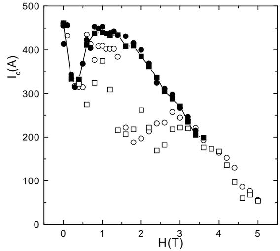
Figure 2: Field dependence of  $I_c$  for carbon-nanotube doped  $MgB_2/Fe$  wire at  $T = 20K$ . Open symbols are obtained with the first current pulse after changing field  $H$  and solid symbols are obtained with second and all subsequent pulses. The round and square symbols are for positive and negative  $H$ , respectively.
