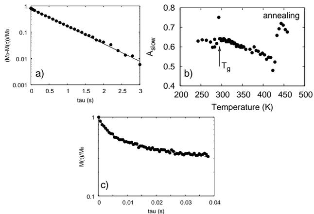
FIG. 2: A typical saturation recovery profile for PPP obtained by 400 MHz  $^1\text{H}$  longitudinal relaxation time measurements at 295K(a) and the temperature dependence of the fraction of the longer relaxation time(b). The shorter fraction was not able to be detected because of slower analog-digital conversion rate than the relaxation rate. A typical decay profile for PPP obtained by 400 MHz  $^1\text{H}$  longitudinal relaxation time measurements in the rotating frame at 295K(c)
