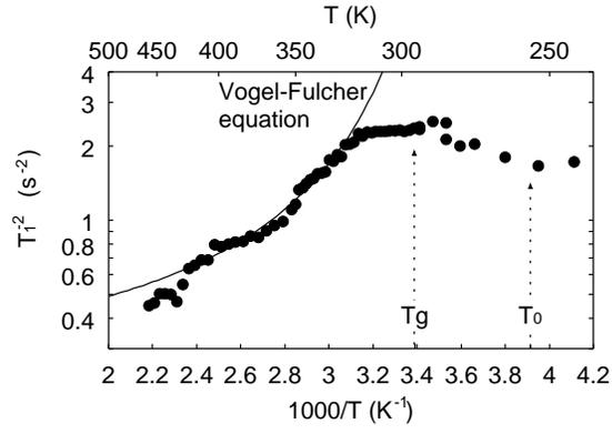
FIG. 5: The plot of 400 MHz  $^1\text{H}$  longitudinal relaxation rate  $(T_1^{-1})^2$  as a function of  $1000/T$ . When one-dimensional diffusion is responsible for the behavior of  $T_1^{-1}$ ,  $(T_1^{-1})^2$  is proportional to  $\tau_c$ .
