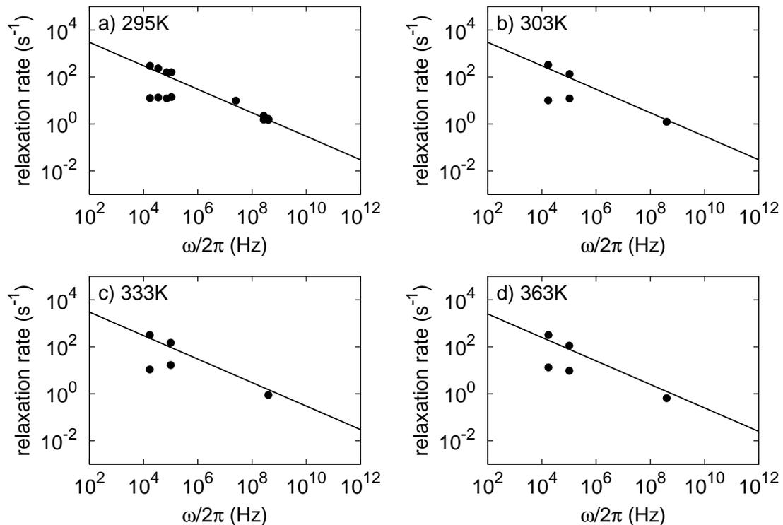
FIG. 4: The frequency dependence of  $^1\text{H}$  longitudinal relaxation rate at 295K (a), 303K (b), 333K (c), and 363K (d). The solid lines of the  $\omega^{-1/2}$  dependence is shown as a guide for eyes.
