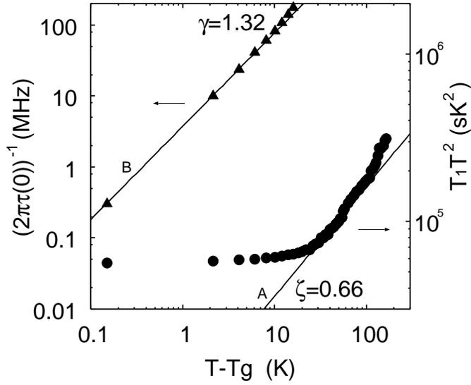
FIG. 6: The plot of  $T_1T^2$  as a function of  $T - T_g$  (right scale). Moreover, the plot of the order-parameter relaxation frequency  $(2\pi\tau(0))^{-1}$  as a function of  $T - T_g$  (left scale).
