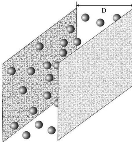
FIG. 1: Schematic representation of our model system: two ideally polarizable planar surfaces with quenched surface charge disorder at separation  $D$  with mobile (point-like) counterions of charge  $Ze_0$  confined in the inter-surface space. The surface charge density is characterized by a Gaussian distribution with fixed mean value of magnitude  $\sigma$  and mean-square deviation  $g$ .
