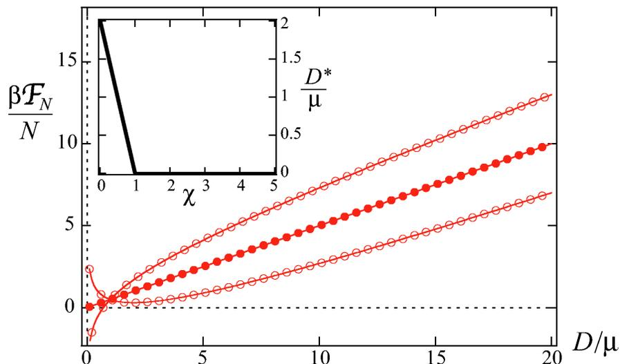
FIG. 2: Free energy per particle, Eq. (72), as a function of dimensionless inter-plate distance  $D/\mu$  for  $\chi = 0, 1$  and  $2$  (bottom line, middle line, top line).  $\mu = e_0/(2\pi\ell_B Z\sigma)$  is the Gouy-Chapman length for mean surface charge density. Inset: dimensionless equilibrium distance  $D^*/\mu$  as a function of the disorder coupling parameter  $\chi$ .
