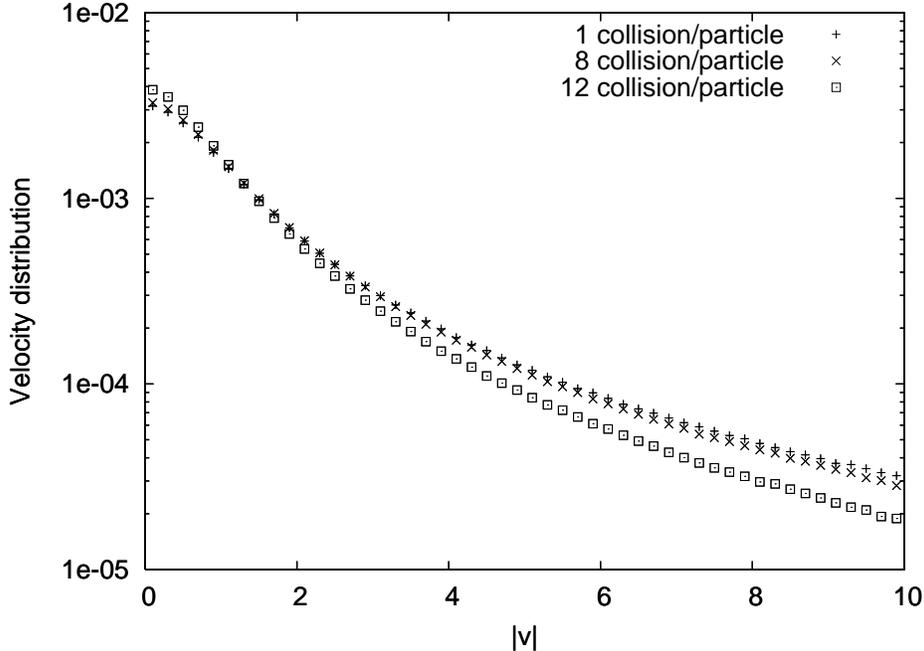
Fig. 1. Evolution of the core of the velocity distribution in log scale. The cutoff length of the Lévy distribution is 10000. The inelasticity is  $\alpha = 0.5$  and the number of particles 10000000. We plot the velocity distribution after 1, 8 and 12 collisions per particle.
