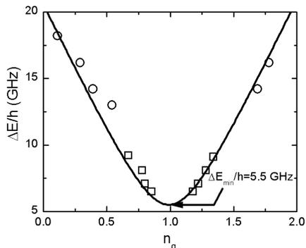
FIG. 4: Energy level separation  $\Delta E$  as a function of  $n_g$  at  $\delta = \pi$ . Squares and circles correspond to one- and two-photon resonances; solid line is a fit with  $E_C/h = 5$  GHz and  $\Delta E_{\min}/h = (E_{J1} - E_{J2})/h = 5.5$  GHz.
