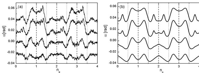
FIG. 3: The same as in Fig. 2 but at a fixed frequency  $\omega/2\pi = 8.2$  GHz with the varied parameter: in experiment (a) being power of excitation (from bottom to top: -75, -63, -49, -42 (dB)) and in theory (b) being amplitude  $\tilde{n}_g$  (from bottom to top: 0.1, 0.2, 0.3, 0.4). Upper curves are shifted.
