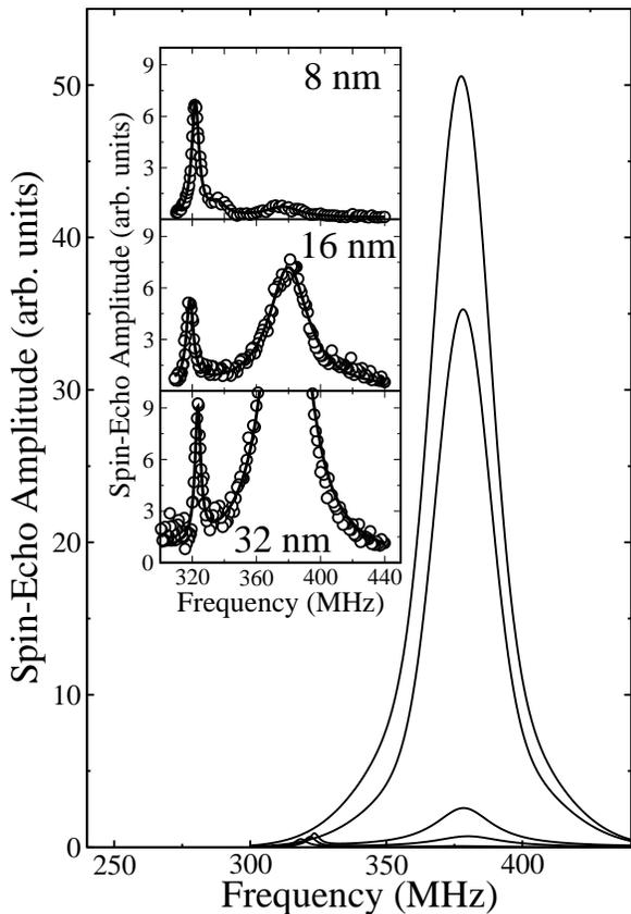
FIG. 1: Zero-field  $^{55}\text{Mn}$  spin-echo amplitude measured at 1.6 K in LSMO/STO films with different thickness.
