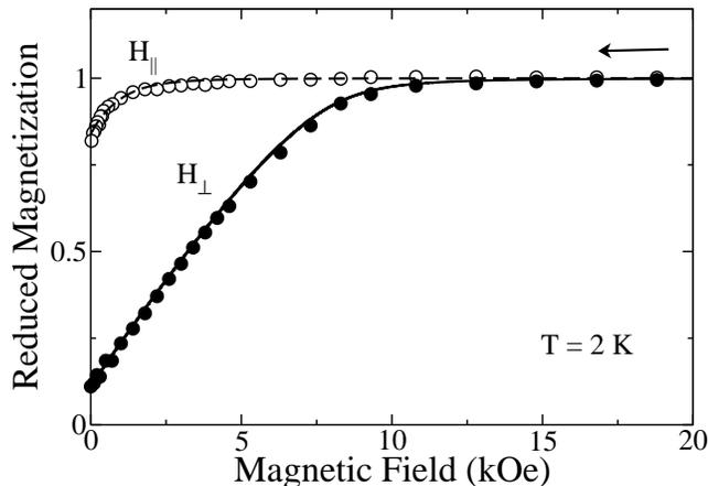
FIG. 8: Field dependence of the reduced in-plane (o) and out-of-plane (●) magnetization at 2 K of the 180 nm thick film. The solid and dashed lines are calculated curves (see text).
