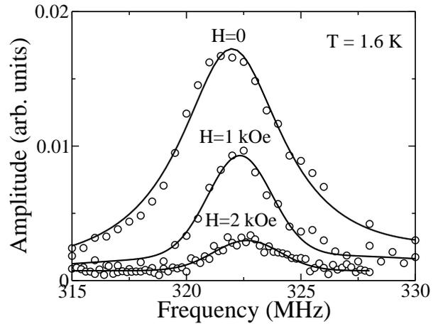
FIG. 7:  $^{55}\text{Mn}$  spin-echo spectra at 1.6 K, corresponding to the insulating region of the LSMO/STO film with thickness of 8 nm, for different values of the dc field applied in the film plane.
