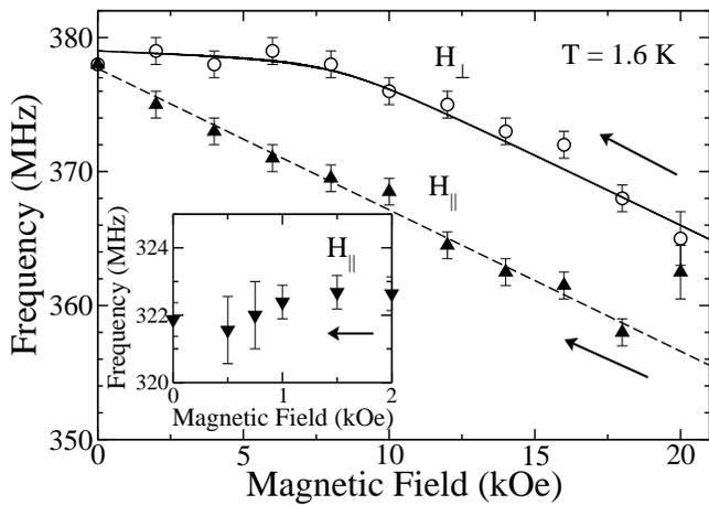
FIG. 3:  $^{55}\text{Mn}$  nuclear resonance frequency  $f^{DE}$  in the 180-nm thick film as functions of the dc field in the film plane ( $\blacktriangle$ ) and perpendicular to the film plane ( $\circ$ ). The solid and dashed lines are calculated curves in the single domain model (see text). The inset shows the shift of the  $f^{4+}$  resonance line in the 8-nm thick film measured with the field applied in the film plane at 1.6 K.
