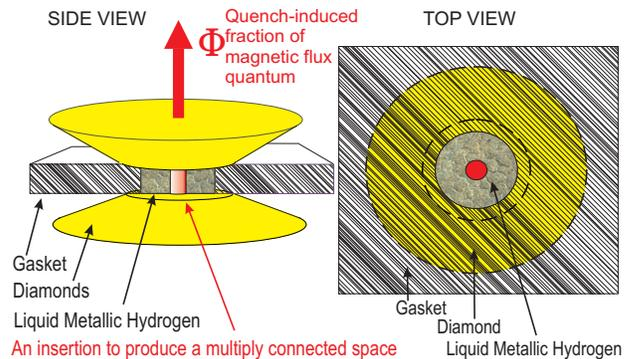
FIG. 1: (Color online) Liquid metallic hydrogen in a high pressure diamond anvil cell. The red insertion makes the sample multiply connected. Thus, a thermal quench should produce  $2\pi \times [\text{integer}]$  winding of the phase of the protonic condensate. This will result in a detectable fractional magnetic flux emitted from the diamond anvil cell. The fraction of the flux quantum will depend on the ratios of superfluid densities of electronic and protonic condensates.
