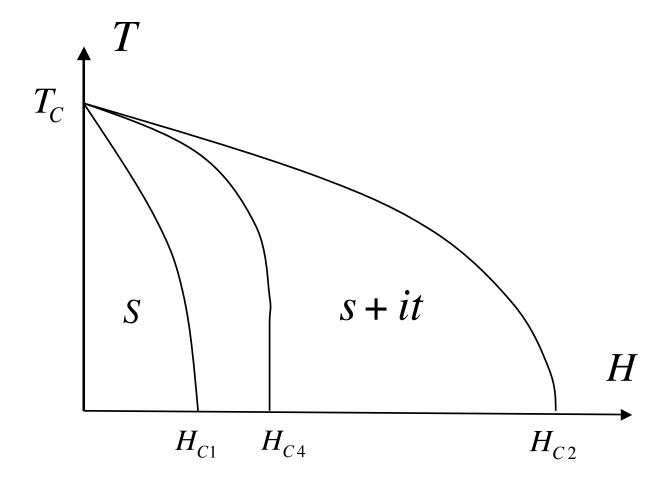
FIG.1: A phase diagram of type-IV superconductor, which is singlet one at H=0 and in M eissner phase,  $0 < H < H_{cl}(T)$ , and characterized by broken inversion and time-reversal symmetries at low temperatures and high magnetic elds,  $H_{c4}(T) < H < H_{c2}(T)$ . In the intermediate region of magnetic elds,  $H_{cl}(T) < H < H_{cl}(T)$ , broken symmetries may be absent or marginal.
