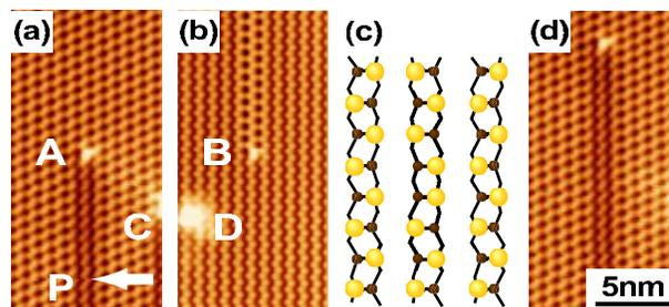
Fig. 1. (color online)(a,b) STM images including topological defects, A, B, which were created on a  $c(4\times 2)$  surface (a), or on a  $p(2\times 2)$  surface (b). Protrusions at C in (a) and D in (b) are impurities as fixed markers. (c) A schematic model of the defect between the two superstructures. (d) STM image after the bias pulse from  $-0.4$  V to  $0.8$  V for 1 sec at P in (a). The STM tip position is fixed during the pulse.
