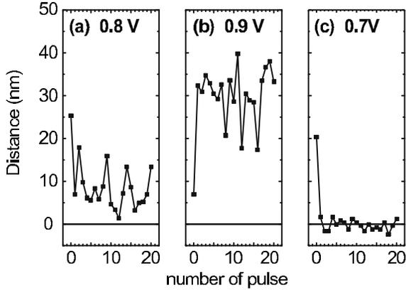
Fig. 2. The distance between the kink and the tunneling point in the dimer-row direction after each bias pulse from  $-0.4$  V to  $0.8$  V (a),  $0.9$  V (b) and  $0.7$  V (c) for 1 sec was applied at the point on the dimer row including the kink. The current during each pulse was  $25$  nA (a),  $33$  nA (b) and  $17$  nA (c).
