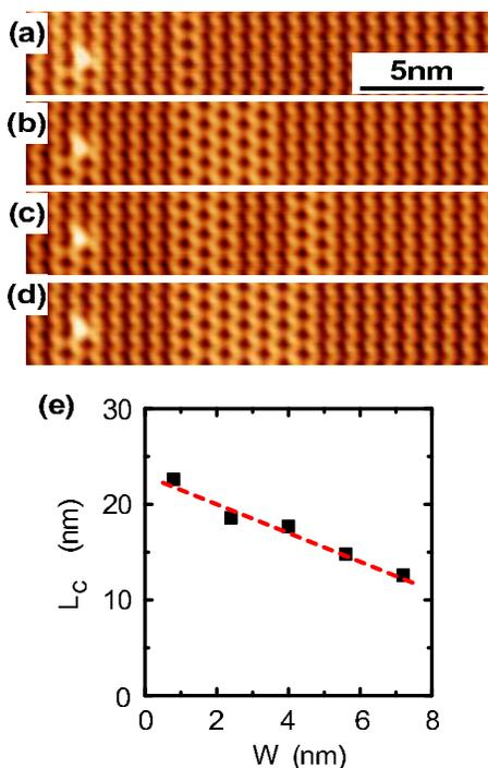
Fig. 4. (color online) (a-d) STM images showing the surfaces with different local structures used for the measurements of the B-type kink motions. The total width of the  $c(4\times 2)$  area,  $W$ , is the same in (b) and (c). (e) The critical distance  $L_c$  in the dimer-axis direction as a function of  $W$ . The slope of the dotted line is  $-1.5$ .
