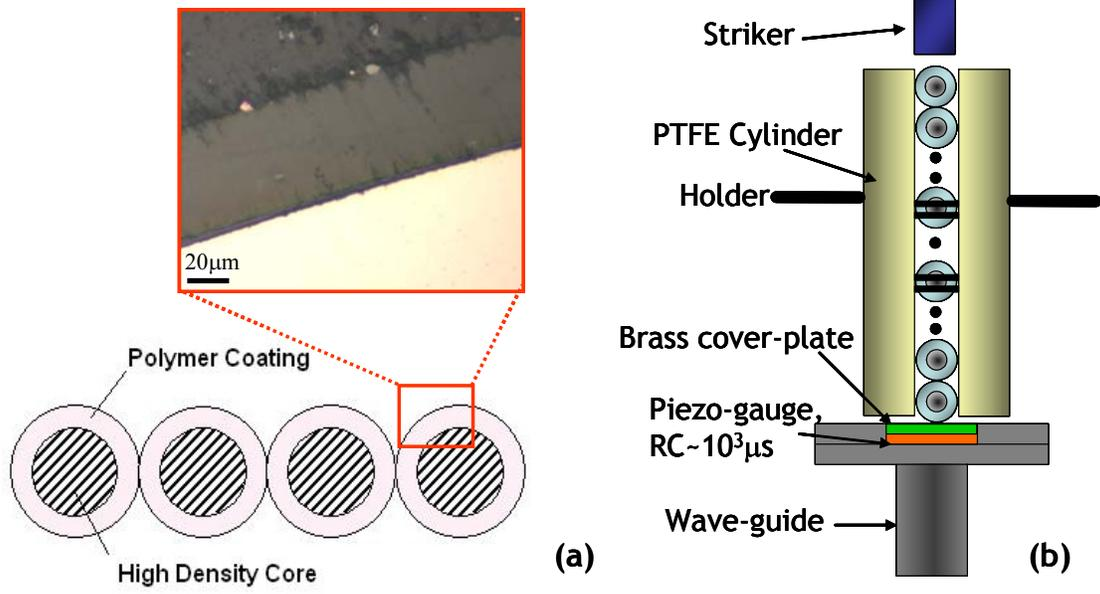
FIG. 2. Experimental set-up for testing of 1-D strongly nonlinear phononic materials. (a) schematic diagram of the chain and optical micrograph showing the Parylene-C polymer coating (b) set up used for the single chain testing, showing the particles with embedded sensors.
