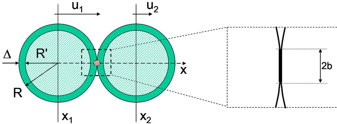
FIG. 1. Schematic diagram showing the contact interaction area between two Parylene coated particles. The inset shows an enlargement of the contact interaction area.
