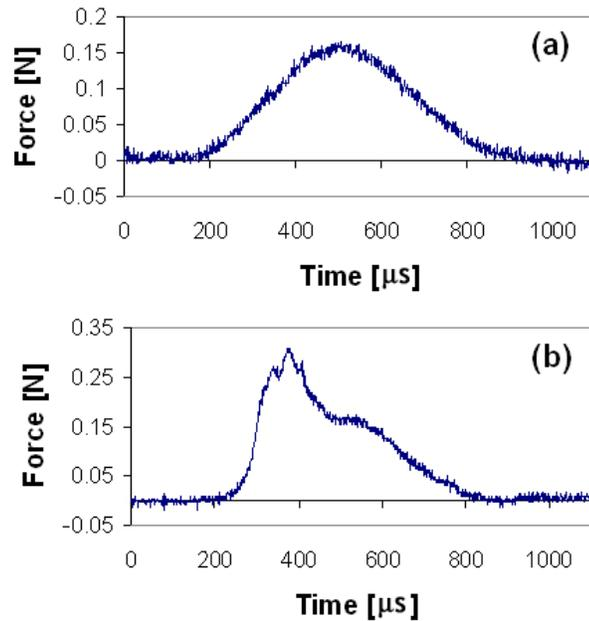
FIG. 6. Pulse generated by a single solitary wave (a) and the shock like nonstationary pulse (b) detected on the wall supporting a chain of 22 smaller ParyleneC balls (2.48 mm diameter,  $m=0.04$  g). (a) Impact at velocity 0.89 m/s with a 2 mm diameter steel ball
