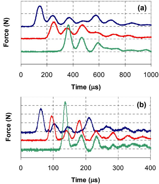
FIG. 5. Train of solitary waves generated in a 21 particles chain composed of (a) Parylene-C coated steel balls (4.86 mm diameter) chain and (b) bare stainless steel beads (4.76 mm diameter) chain for comparison. Sensors are placed in the 9<sup>th</sup> ball from the bottom (top curve), 5<sup>th</sup> ball from the bottom (middle curve) and at the bottom wall. The velocity of striker (1.23 g Al<sub>2</sub>O<sub>3</sub> cylinder) was 0.44 m/s. Y-axis scale is 1 N for (a) and 5 N for (b).
