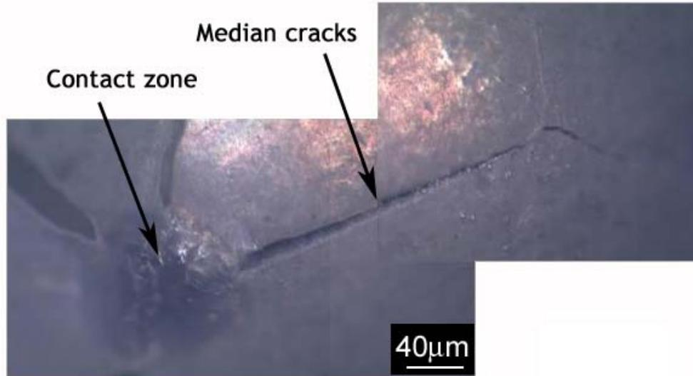
FIG. 7. Typical four median cracks originating away from the deformed contact zone observed after high amplitude dynamic testing with a maximum force on the level of  $\sim 3$  N. Note that they appear before the Hertzian ring cracks which are supposed to originate on the outside area of the contact zone.
