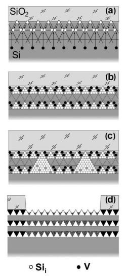
FIG. 1. A scheme of self-assembled silicon quantum wells confined by the  $\delta$  - barriers heavily doped with boron on the Si (100) surface.
