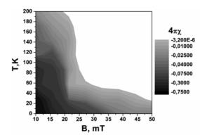
FIG. 5. Plots of static magnetic susceptibility vs temperature and magnetic field that was observed under conditions of field-in cooling in the B-doped silicon nanostructure. These data can be used visually to define  $H_{cl}$ ,  $H_{cl}$ =215 Oe.
