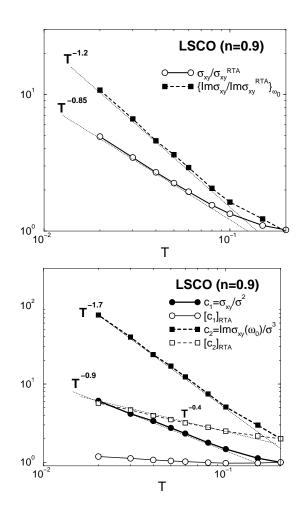
FIG. 9: (a)  $\sigma_{xy}/\sigma_{xy}^0 \propto T^{-0.85}$  at  $\omega = 0$  and  $\mathrm{Im}\sigma_{xy}/\mathrm{Im}\sigma_{xy}^0 \propto T^{-1.2}$  for small  $\omega_0$ . This result suggests that they are proportional to  $\xi^2$  and  $\xi^3$  ( $\xi$  being the AF correlation length) for  $T = 0.03 \sim 0.1$ . (b)  $\sigma_{xy}/\sigma^2 \propto T^{-0.9}$  at  $\omega = 0$  and  $\mathrm{Im}\sigma_{xy}/\sigma_{xy}^3 \propto T^{-1.7}$  for small  $\omega_0$ .
