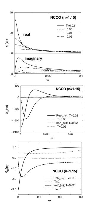
FIG. 16: Obtained  $\sigma(\omega)$ ,  $\sigma_{xy}(\omega)$  and  $R_{\rm H}(\omega)$  for NCCO by the CVC-FLEX approximation.
