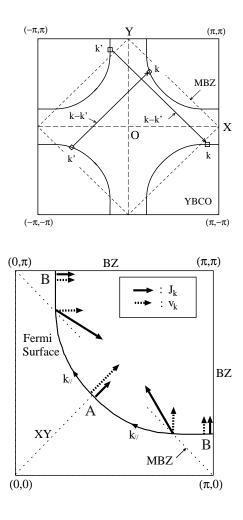
FIG. 1: Schematic **k**-dependences of  $\mathbf{J}_{\mathbf{k}}$  and  $\mathbf{v}_{\mathbf{k}}$  when the AF fluctuations with  $\mathbf{Q} \approx (\pi, pi)$  are strong. The cold-spot on the Fermi surface for hole-doped (electron-doped) systems exist around A (B).
