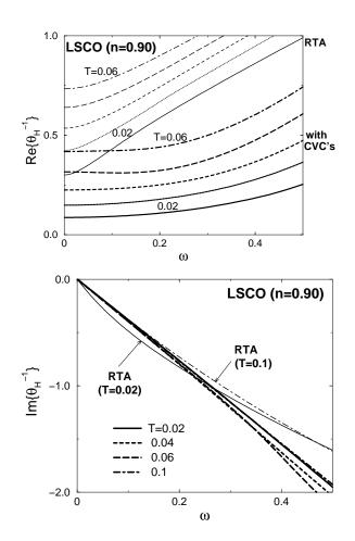
FIG. 11: Obtained  $\omega$ -dependence of the inverse Hall angle for several temperatures. We see that  $\text{Re}\theta_{\text{H}}^{-1}$  is approximately  $\omega$ independent for  $\omega < 0.2$  while it's temperature dependence is large. This result, obtained by taking the CVC into account, is consistent with experiments.
