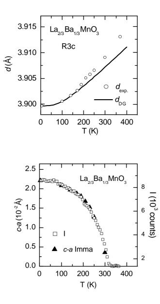
Fig. 8. Temperature dependences of the Mn-Mn distance d for the  $R\overline{3}c$  crystalline phase of the La<sub>2/3</sub>Ba<sub>1/3</sub>MnO<sub>3</sub> compound (upper panel, circles depict the experimental data and the solid line depicts the Debye-Grüneisen curve), of the *c-a* difference for the *Imma* phase and of the integrated intensity *I* of magnetic Bragg peak (triangles and squares, respectively; lower panel). Error bars are of the experimental points sizes approximately.
