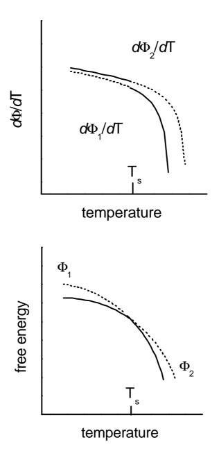
Fig. 7. Temperature dependences of the Gibbs free energies of the high temperature  $(\Phi_1)$  and low temperature  $(\Phi_2)$  phases (lower panel) and their temperature derivatives (upper panel) at the first order phase transition. Solid line corresponds to the thermodynamically equilibrium state,  $T_s$  indicates the transition temperature.
