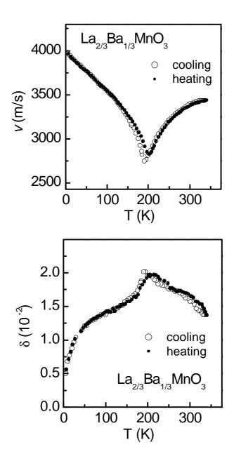
Fig. 1. Temperature dependences of the sound velocity v (upper panel) and logarithmic decrement  $\delta$  (lower panel) of the La<sub>2/3</sub>Ba<sub>1/3</sub>MnO<sub>3</sub> manganite when cooling (o) and heating (•). Error bars are of the experimental points sizes approximately.
