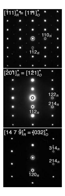
Fig. 10. ED patterns of La<sub>2/3</sub>Ba<sub>1/3</sub>MnO<sub>3</sub> along $[\overline{1}11]_{R}^{*}$ ,  $[\overline{2}01]_{R}^{*}$ , and  $[14\ 7\ 9]_{R}^{*}$  obtained at 300 K (R – rhombohedric phase). These ED patterns also match perfectly with the  $[111]_{O}^{*}$ ,  $[121]_{O}^{*}$  and  $[032]_{O}^{*}$  ED patterns of the *Imma* low temperature phase (O – orthorhombic phase), respectively.
