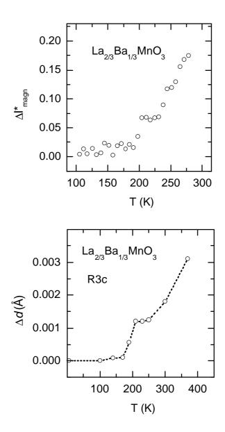
Fig. 9. The first order phase transition contributions  $\Delta I^*_{magn}$  (to the integrated intensity *I* of magnetic Bragg peak, upper panel), and  $\Delta d$  (to the Mn-Mn distance *d* in the  $R\overline{3}c$  crystalline phase, lower panel) of the La<sub>2/3</sub>Ba<sub>1/3</sub>MnO<sub>3</sub> compound. Dotted line is guide to the eyes, error bars are of the doubled experimental points sizes approximately.
