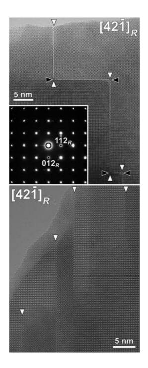
Fig. 11. Room temperature HREM images along the  $[42\overline{1}]$  zone. Note the presence of planar defects running along the  $\{012\}$ - and  $\{1\overline{1}2\}$ -type planes (indicated by arrowheads). The corresponding ED pattern of the top HREM image is shown as an inset.
