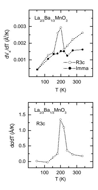
Fig. 4. Temperature derivatives of the volume  $V_a$  per manganese atom for the  $R\overline{3}c$  and *Imma* phases (upper panel), and of the *c* parameter (doubled Mn-Mn distance *d*) of the  $R\overline{3}c$  crystalline phase (lower panel) in the La<sub>2/3</sub>Ba<sub>1/3</sub>MnO<sub>3</sub> compound. Dotted lines are guides to the eyes, error bars are of the experimental points sizes approximately.
