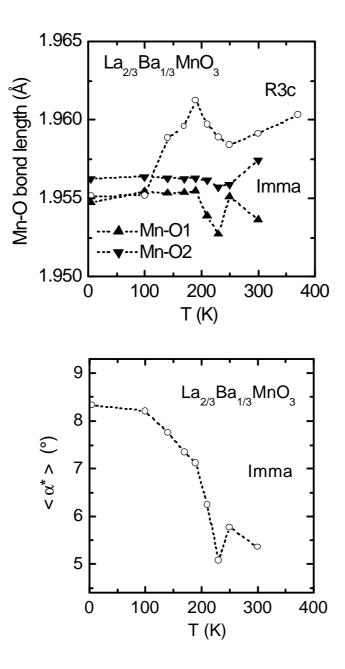
Fig. 6. Mn-O bond lengths as a function of temperature for rhombohedral  $R\overline{3}c$  (circles) and orthorhombic *Imma* ( $\blacktriangle$ - Mn-O1,  $\nabla$ - Mn-O2) phases of La<sub>2/3</sub>Ba<sub>1/3</sub>MnO<sub>3</sub> (upper panel); average deviation from 180° of the Mn-O-Mn bond angle for the *Imma* phase  $<\alpha^*>=180^\circ-(\alpha_1+2\alpha_2)/3$  (lower panel). Dotted lines are guides to the eyes, error bars are of the experimental points sizes approximately.
