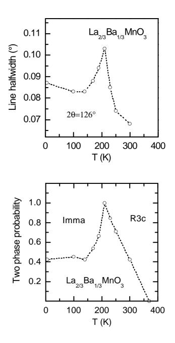
Fig. 3. Temperature dependences of the line halfwidth for the diffraction angle  $2\theta=126^{\circ}$  for the  $R\overline{3}c$  and *Imma* phases (upper panel), and of the normalized probability of the simultaneous presence of the two phases in the La<sub>2/3</sub>Ba<sub>1/3</sub>MnO<sub>3</sub> compound (lower panel). Dotted lines are guides to the eyes, error bars are of the experimental points sizes approximately.
