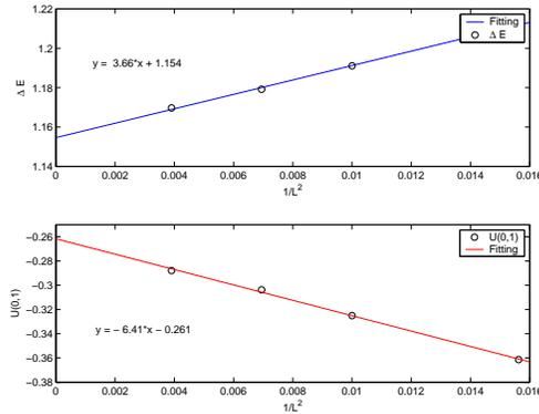
Fig. 5 – (Color online) The finite size scaling of  $\Delta E$  and  $U(0, 1)$  in an  $L \times L$  lattice. The impurity quantities  $\Delta E$  and  $U(0, 1)$  converge with  $1/L^2$  and are derived as a difference of extensive quantities and therefore have larger errorbars.
