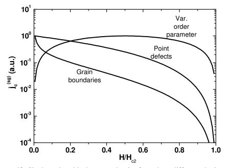
**Figure 10.** Single grain critical current density from three different pinning mechanisms (grain boundaries, point defects and variations of the superconducting order parameter) as a function of the reduced field  $H/H_{c2}$ . The curves are normalized to the respective maximum values.
