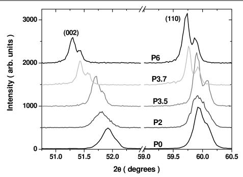
**Figure 1.** X-Ray diffraction patterns on (002) and (110) reflections for unirradiated (P0) and irradiated (P2, P3.5, P3.7, P6) samples.
