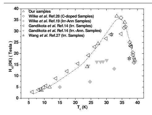
**Figure 7.** Upper critical field as a function of critical temperature in irradiated or C-doped samples (open symbols) and in irradiated and then annealed samples (full symbols); the line is only a guide for eyes.
