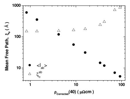
**Figure 12.** In-plane BCS coherence length  $\xi_0$  for the  $\sigma$ -band (open symbols) and in-plane mean free path (solid symbols) as a function of corrected residual resistivity.
