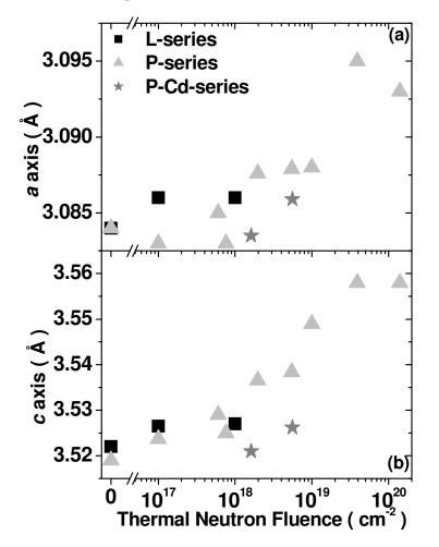
**Figure 2.** *a* and *c* axes as a function of thermal neutron fluence for L- (black squares), P- (grey triangles) and P-Cd-series (grey stars).
