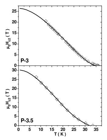
Figure 8. Upper critical field data (open symbols) and H<sub>c2</sub> fit curves (solid lines) for P3 and P3.5 samples.
