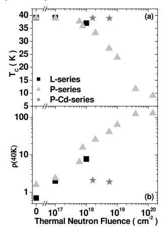
Figure 4. (a) Critical temperature  $T_c$  and (b) resistivity at 40 K,  $\rho(40K)$  as a function of thermal neutron fluence.
