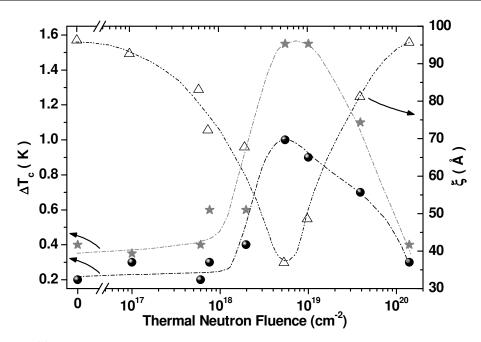
**Figure 11.** Transition width  $\Delta T_c$  ( $T_{90\%}$  -  $T_{10\%}$ , black circles,  $T_{98\%}$  -  $T_{2\%}$ , grey stars) and coherence length  $\xi$  (open symbols) as a function of thermal neutron fluence: the lines are guides for eyes.
