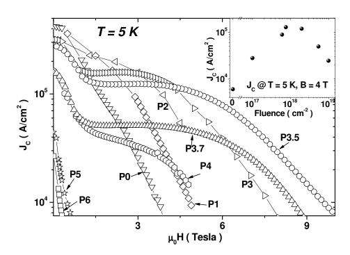
**Figure 9.** In the main panel, critical current density at 5 K as a function of magnetic field and as a function of fluence at 4 T, in the inset.
