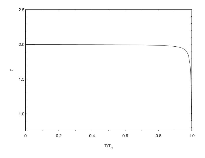
Figure(2). The ratio of upper critical field ( $\gamma = \frac{H_{c2}^{//ab}}{H_{c2}^{//c}}$ ) of the results of H<sub>c2</sub> in Figure.(1) versus temperature .
