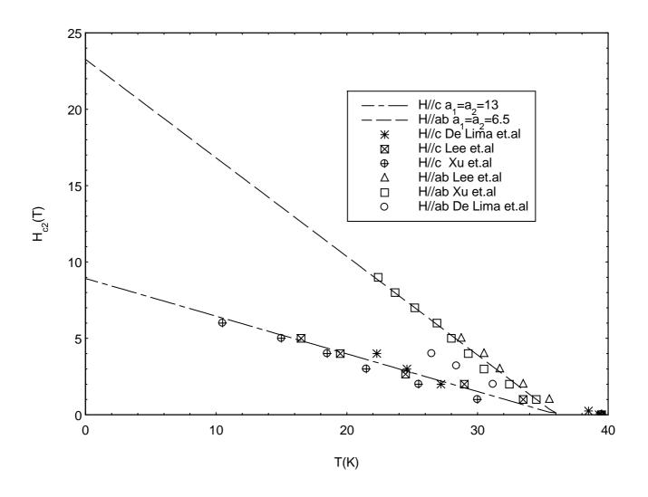
Figure(1). We fit Eq.(12) to the experimental data of upper critical field of single crystal MgB<sub>2</sub>[21-23] and find the upper critical field in ab-plane( $H_{c2}^{/\prime ab}$ ),  $H_{c2}^{\prime\prime ab} = H_{c2}$ (6.5,6.5,0.7,0.5), and in c-axis  $(H_{c2}^{\prime\prime c})$ ,  $H_{c2}^{\prime\prime c} = H_{c2}$ (13,13,0.7,0.5).
