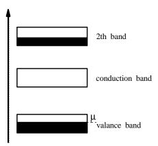
FIG. 3: Energy bands for a laser phase of a semiconductor where  $\mu$  denotes the chemical potential. Here, both the valance and 2th bands are partially filled, the population is inverted between the 2th and conduction bands.
