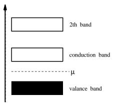
FIG. 1: Energy bands for the normal (positive-temperature) phase of a semiconductor where  $\mu$  denotes the chemical potential.
