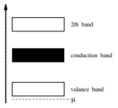
FIG. 2: Energy bands for a partially negative-temperature phase of a semiconductor where  $\mu$  denotes the chemical potential. Here, the population is inverted between the valance and conduction bands.
