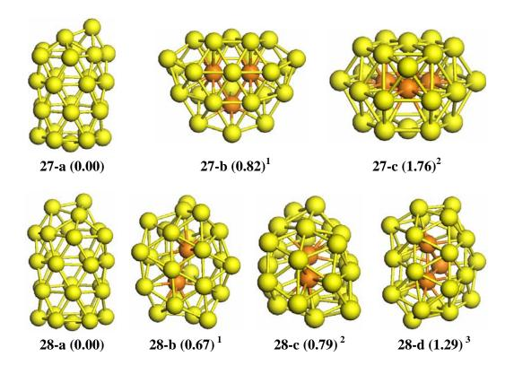
FIG. 3. (Color online) Structures of  $Au_{27}$  and  $Au_{28}$ . The values in the parentheses are the relative energies (in unit of eV) to those of the tube-like structures. <sup>1</sup>See Ref. 8; <sup>2</sup>See Ref. 9; <sup>3</sup>See Ref. 10.
