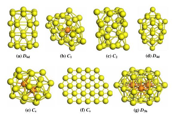
FIG. 1. (Color online) Optimized ground state (a) and selected low-lying isomers (b-g) of Au<sub>26</sub>.
