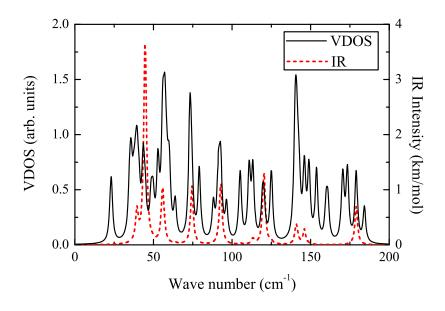
FIG. 2. (Color online) The VDOS and corresponding FIR absorption spectrum of the lowest-energy tube-like Au<sub>26</sub>, shown by the solid and dashed line, respectively.
