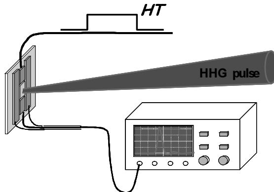
Figure 1 : principle of the TPC measurements
