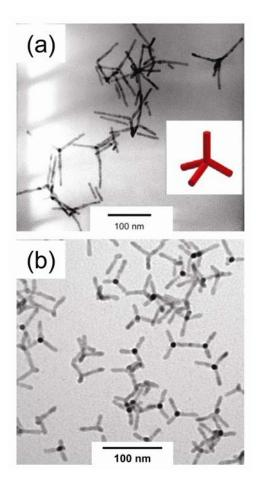
**Figure 1:** TEM images of CdTe tetrapods with different size; (a) large TPs with 12 nm / 80 nm arm diameter and length; (b) small TPs with 7 nm / 30 nm arm diameter and length. The inset shows a schematic drawing of a tetrapod.
