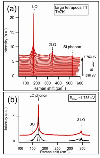
**Figure 3:** (a) Resonant Raman spectra of large CdTe tetrapods at T = 7 K. (b) a spectrum in resonant condition (red line) and Lorentz fits to the data (black dotted lines). We observe a mode at 148 cm<sup>-1</sup> (FWHM = 1.2 cm<sup>-1</sup>), a mode at 173.5 cm<sup>-1</sup> (FWHM = 1.5 cm<sup>-1</sup>) and a broad underlying signal that was fitted with a peak at 170 cm<sup>-1</sup> (FWHM = 14 cm<sup>-1</sup>). Experimental spectra have been shifted for clarity.
