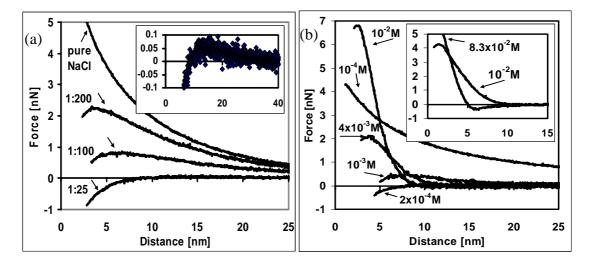
Fig. 2a- Force vs. distance curves for pure NaCl and three  $Co(NH_3)_6Cl_3$ : NaCl mixtures. The ionic strength in all cases was set to give  $r_{DH} = 10nm$ . The pH was set to 6 by negligible titrations of either HCl or NaOH. Inset- a magnified view of the 1:25 mixture.
