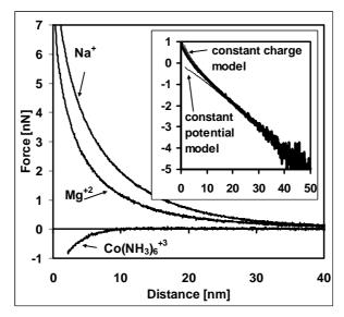
Fig. 1- Force vs. distance curves for three different cations and the same Cl<sup>-</sup> anion. The ionic strength in all cases corresponds to  $r_{DH} = 10nm$ . The pH was set to 6 by negligible addition of HCl or NaOH. Inset- Semilog plot of the force vs. distance for the NaCl curve together with best fit to PB models with constant charge or constant surface potential.
