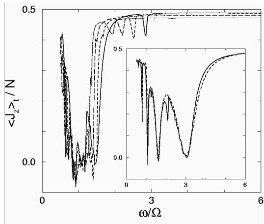
FIG. 4: Time-averaged population imbalance  $\langle J_z \rangle_t / N$  for the driven Bosonic Josephson junction with  $N = 100$  particles, tilt  $2\mu_0/\Omega = 3.0$ , and one-photon resonant driving frequency  $\omega/\Omega = 3.0$ . The interaction parameters are as in Fig. 2.
