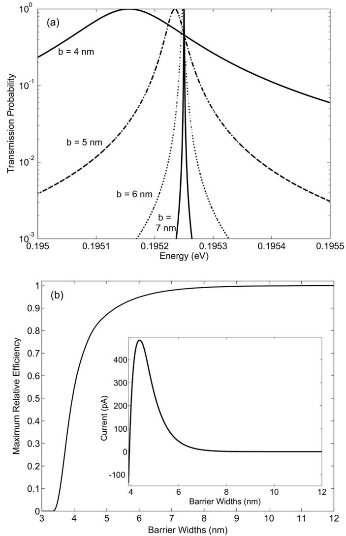
**Figure (4)** (a) The width of resonances for  $w = 7$  nm and  $b = 4, 5, 6$  and  $7$  nm (see figure 1). (b) Device efficiency relative to the Carnot value  $\eta_c = (1-1K/10K) = 90\%$  versus  $b$  for  $w = 7$  nm. For each value of  $b$ ,  $\mu_C$  and  $V_{bias}$  have been tuned to find the maximum efficiency value. (Inset) Device current (sampled at  $-1$  mV) versus  $b$ .
