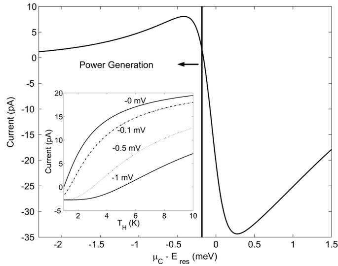
**Figure 6.** The device current sampled at  $V_{bias} = -1$  mV versus the difference between the fixed resonance energy and varied electrochemical potential. (Inset) Current, sampled at  $V_{bias} = 0$  mV,  $-0.1$  mV,  $-0.5$  mV and  $-1$  mV as labeled, versus the hot reservoir temperature.  $\mu_C - E_{res} = -0.3$  meV, which corresponds to the electrochemical potential for maximum efficiency as shown in figure 5.
