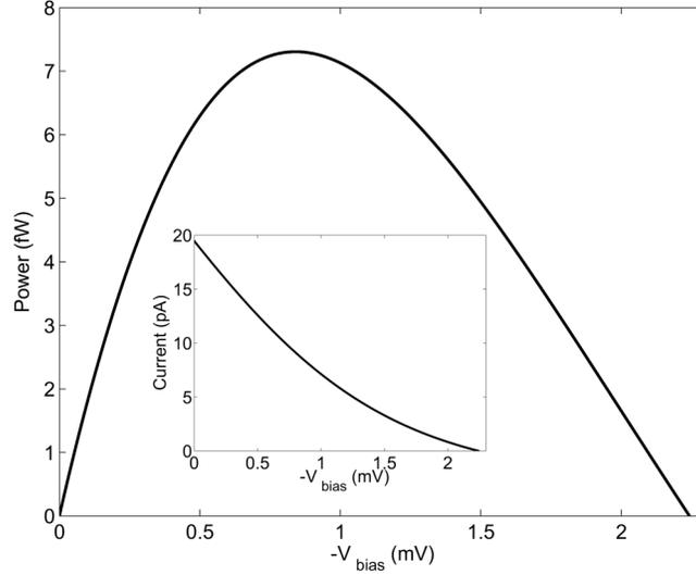
**Figure 7.** Power versus bias voltage. (Inset) Current versus the bias voltage.  $\mu_C - E_{res} = -0.3$  meV.
