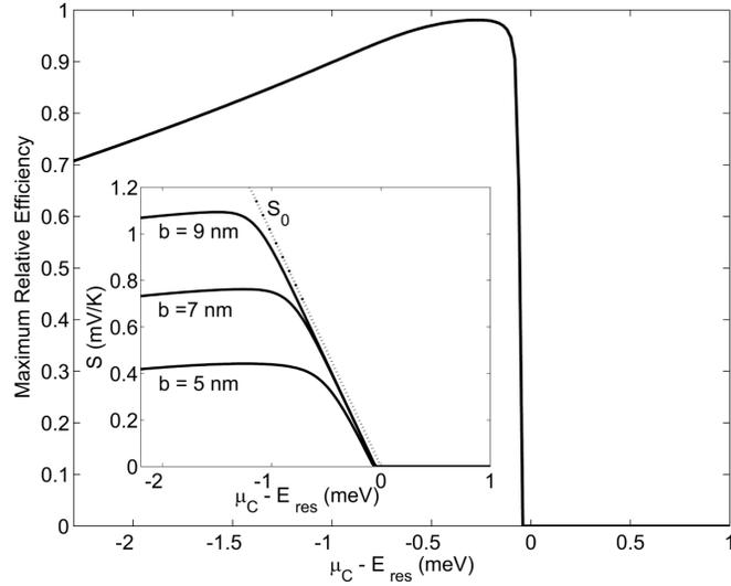
**Figure 5.**  $\eta/\eta_c$  as a function of,  $\mu_C$  with fixed  $E_{res}$ . (Inset) The Seebeck coefficient,  $S$ , as a function of  $\mu_C$  with fixed  $E_{res}$  for different barrier widths as labeled. The maximum possible Seebeck coefficient, which is associated with reversibility,  $S_0$ , is also included.
