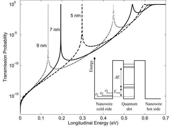
**Figure 3.** The transmission probabilities for double barrier structures with  $b = 20$  nm and  $w = 5$  nm, 7 nm and 9 nm. (Inset) Longitudinal energies,  $E_{res}$  and  $E_{res} + \Delta E$ , are quantized due to the double barrier structure and transverse energies,  $\epsilon_{1,2,3}$ , due to the dimensions of the nanowire (adapted from reference [6]).
