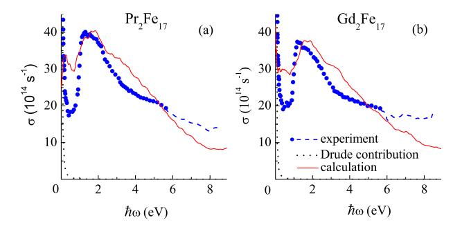
FIG. 2: (Colouronline) Experim ental (dark circles and dashed lines) and calculated (solid lines) dispersion dependencies of optical conductivity for  $Pr_2Fe_{17}$  (a) and  $Gd_2Fe_{17}$  (b) compounds. Dashed lines represent (!) values obtained by K ram ers-K ronig transformation from rejection spectra. Doted lines correspond to intraband contributions estimated by D rude formula. Calculated values are in arbitrary units.
