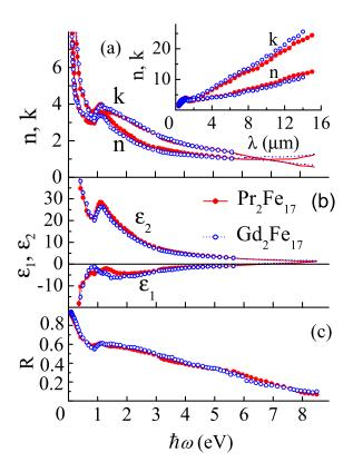
FIG. 1: (Colour online) Experim entaloptical constants n and k (panela), dielectric functions  $_1$  and  $_2$  (panelb), and reectivity spectra R (panelc) for PrFe $_1$ 7 (full circles and solid line) and G d $_2$ Fe $_1$ 7 (empty circles and doted line) compounds. Doted and solid lines above 5.6 eV represent values obtained by K ramers-K ronig transformation from reection spectra. Inset presents dependences of the optical constants on wavelength for an expanded view in infrared region.
