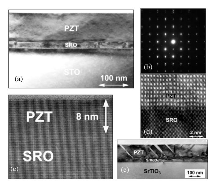
**Figure 2.** Transmission electron microscopy investigations of the PbZr<sub>0.2</sub>Ti<sub>0.8</sub>O<sub>3</sub>/ SrRuO<sub>3</sub>/SrTiO<sub>3</sub> heterostructures. The images are: (a) cross-section TEM micrograph of a defect-free PZT film (t= 90 nm) on top of a SRO film (t= 20 nm) grown on vicinal STO (001) and (b) electron-diffraction pattern of this heterostructure; (c) HRTEM micrograph of an ultrathin PZT film (8nm); (d) Z-contrast STEM
