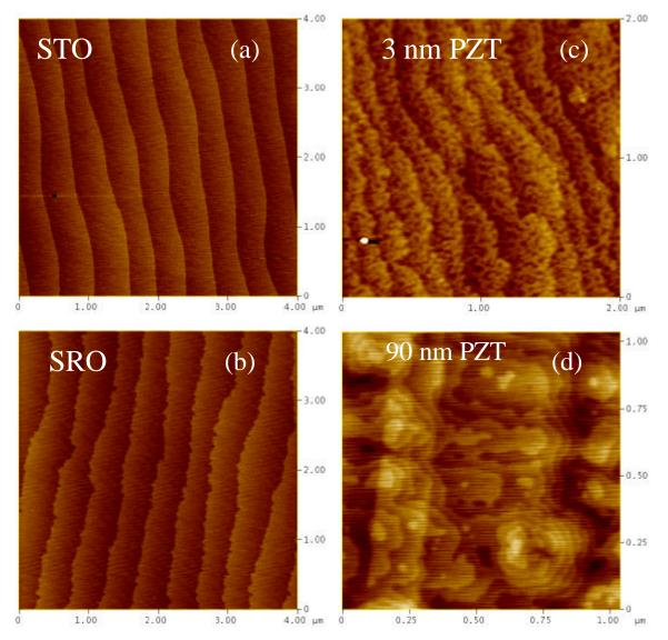
**Figure 1**. AFM images of the vicinal  $SrTiO_3$  substrate and the eptaxially PLD-grown  $SrRuO_3$  and  $PbZr_{0.2}Ti_{0.8}O_3$  layers. The one-unit-cell stepped terraces (400 nm width) of a  $SrTiO_3$  substrate are visible in (a). The morphology of the  $SrRuO_3$  step-flow grown (t= 20 nm) on this substrate is shown in (b). In (c) and (d) the morphology of
