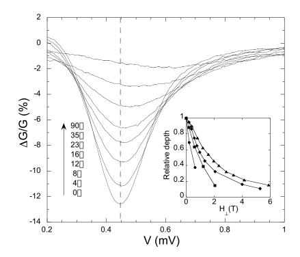
FIG.2: Pairing resonance at several eld orientations for a g = 5.6 lm at 60 mK in a eld of 5.9 T. = 0 corresponds to eld parallel to the lm plane. The vertical dashed line marks the position of the parallel eld resonance. Inset: the relative depth of the PR as a function of the perpendicular component of magnetic eld for several lm conductances: Circle g = 58, Square g = 26, D iam ond g = 12, Triangle g = 5.6.
