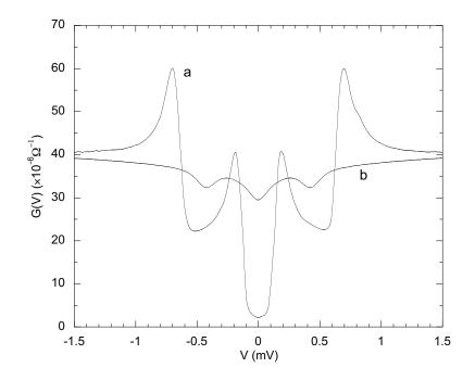
FIG.1: Tunneling conductance of a g = 12 lm at 60 mK in superconducting and normal states, where parallel elds are 4.5 T (a) and 5.7 T (b), respectively. In the superconducting state, the Zeem an split of BCS DOS manifests itself as two peaks of tunneling conductance on either side of V = 0.
