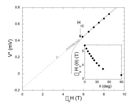
FIG. 3: The position of the PR as a function of magnetic eld for the g = 5.6 lm at 60 mK. The vertical arrow marks the parallel critical eld. Solid symbols correspond to parallel eld. The open symbols were taken at = 8;12;16;19;23;29;45; and 90 (from right to left). The dashed line is provided as a guide to the eye. The solid line is a tofEq. 1) to the parallel eld data. The inset shows the critical eld as a function of tilt angle.
