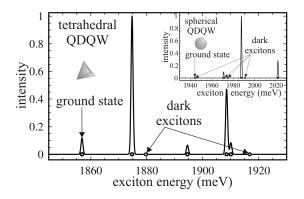
Fig.1. Normalized intensities of the lowest exciton levels in the optical absorption spectrum of a tetrahedral QDQW (the insert gives the intensities for a spherical QDQW). Spectral lines are broadened by a Gaussian to enhance visualization.
