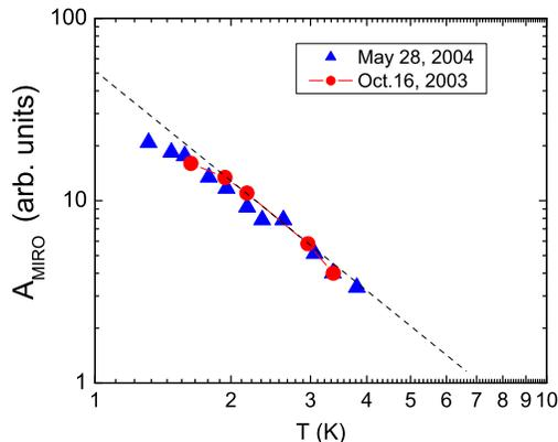
FIG. 4: (Color online) Temperature dependence of MIRO amplitude in a high-mobility GaAs/AlGaAs sample in arbitrary units determined by fitting experimental traces with eq. (1) using  $\Gamma$  and  $A$  as fitting parameters. Results of  $\Gamma(T)$  dependence were published in Ref. 16.
