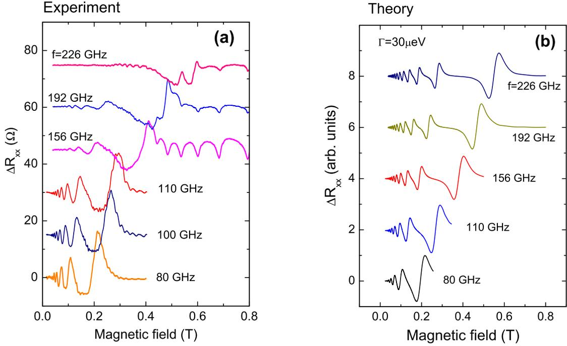
FIG. 1: (Color online) MIRO ( $\Delta R_{xx} = R_{xx}(\text{MWs on}) - R_{xx}(\text{no MWs})$ ) for different MW frequencies from 80 to 226 GHz: (a) experimental traces at  $T=1.8\text{K}$ , (b) corresponding normalized theoretical traces by eq. (1) with the same Landau level width  $\Gamma=30 \mu\text{eV}$ . Traces are shifted vertically for clarity.
