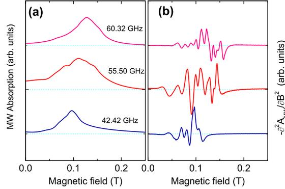
FIG. 5: (Color on line) **(a)** Examples of the microwave magneto-absorption spectra measured in EPR resonator on a rectangular 2DEG sample,  $w=1.0$  mm; **(b)** the second derivative of the corresponding spectra.
