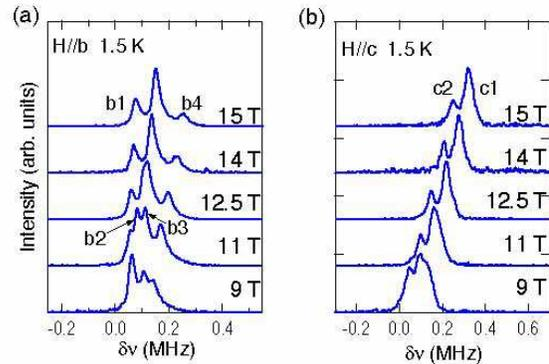
FIG. 2:  $^{77}\text{Se}$  NMR spectra at  $T = 1.5$  K for the external field along the  $b$ -axis (a) and along the  $c$ -axis (b). The resolved four (two) peaks are denoted as  $b_1, b_2, b_3,$  and  $b_4$  ( $c_1$  and  $c_2$ ).
