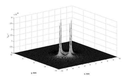
Fig. 2a. Effective potential in the Ioffe-Pritchard trap produced by the DC ring and DC bar currents (z=0).
