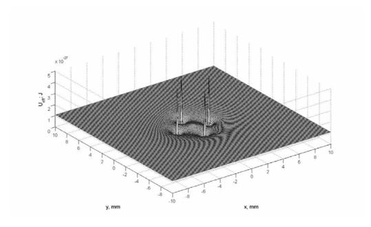
Fig. 2b. Multi-minimum effective potential at the centre of the trap (z=0) of the Ioffe-Pritchard trap fed by the RF and DC currents
