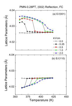
Figure 7. Lattice parameter as a function of temperature derived from the (002)-reflection of PMN-0.28PT under different electric field levels applied along: (a) E//[001], and (b) E//[110].
