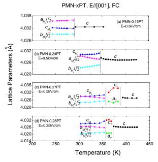
Figure 3. Lattice parameters as a function of temperature for [001] field cooled PMN-xPT crystals: (a) PMN-0.15PT, E=0.5kv/cm; (b) PMN-0.24PT, E=0.5kv/cm; (c) PMN-0.27PT, E=0.5kv/cm; and (d) PMN-0.28PT under E=0.25kv/cm.
