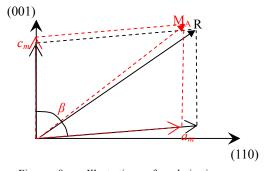
Figure 8. Illustration of polarization vectors of the rhombohedral (R) and monoclinc  $M_A$  (Cm) phases, represented with same monoclinic angle  $\beta$  in the HHL zone of reciprocal space. The R unit cell can be expressed in terms of a monoclinic one by:  $a_m = 2a_r \cos(\alpha/2)$ ,  $b_m = 2a_r \sin(\alpha/2)$ ,  $a_m = a_r$ ,  $\cos(\beta) = (1-2\sin^2(\alpha/2))/\cos(\alpha/2)$ , where  $a_r$  and  $\alpha$  are the R3m cell parameters.
