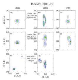
Figure 4. Mesh scans taken about the pseudocubic (002), (220) and (200) reflections for [001] field cooled PMN-xPT crystals: (a) PMN-0.15PT, E=0.5kV/cm at 270K; (b) PMN-0.35PT, E=2kV/cm at 300K; and (c) PMN-0.38PT, E=3kV/cm at 243K.
