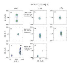
Figure 6. Mesh scans taken about the pseudocubic (002), (220) and (200) reflections for [110] field cooled PMN-xPT crystals: (a) PMN-0.15PT, E=0.5kV/cm at 253K; (b) PMN-0.35PT, E=2kV/cm at 300K; and (c) PMN-0.38PT, E=3kV/cm at 243K.
