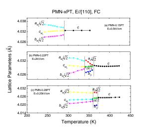
Figure 5. Lattice parameters as a function of temperature for [110] field cooled PMN-xPT crystals: (a) PMN-0.15PT, E=0.5kv/cm; (b) PMN-0.22PT, E=2kv/cm; and (c) PMN-0.28PT, E=0.25kv/cm.
