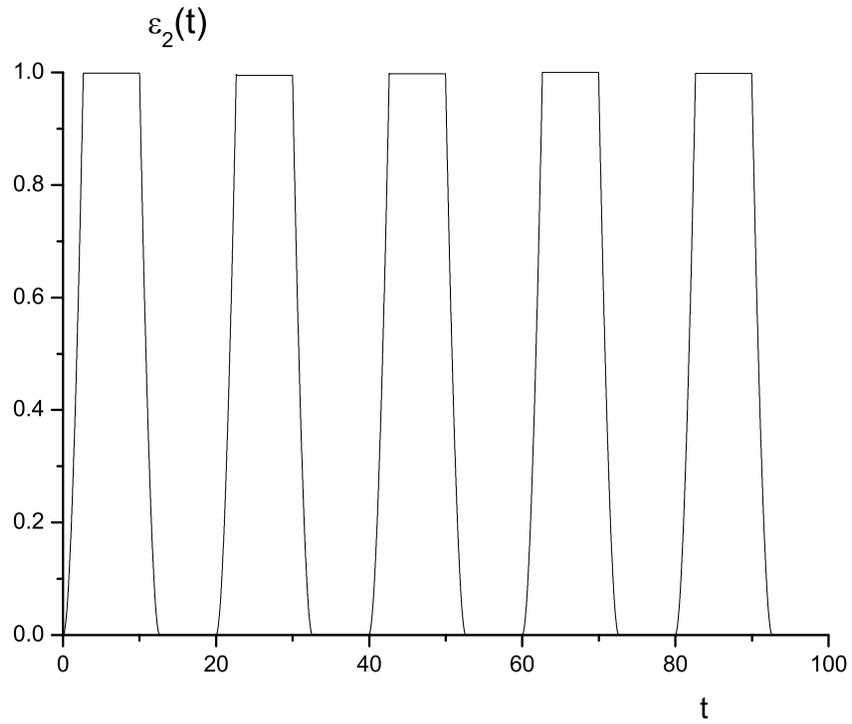
FIG .5. Regulated equidistant pulses of  $\epsilon_2(t)$ , formed by switching on and off the resonant field, with  $b = 0.7$ , so that  $\epsilon_2(t)$  equals one during the time intervals  $t = 7.35$  (in units of  $\tau^{-1}$ ), and it equals zero during the same intervals  $t = 7.35$ .
