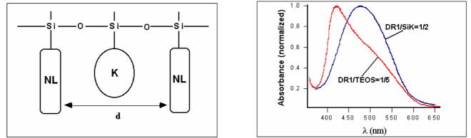
Figure 2. The carbazole units act as spacer between the NLO chromophore thus reducing their mutual interactions. Their effect on the absorption spectra is quite clear (see material preparation section for nomenclature).
