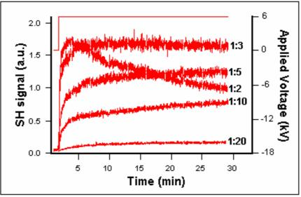
Figure 7. Comparison among the poling samples dynamics with different DR1 concentrations.
