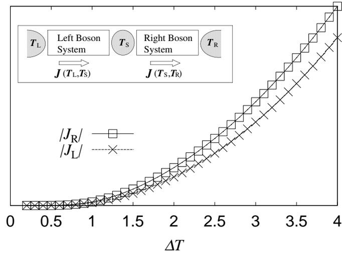
Fig. 3. Simple explanation of asymmetric heat flow using phonon reservoirs with temperatures  $T_L$ ,  $T_S$ , and  $T_R$ . The temperature  $T_S$  is determined by the condition  $J(T_L, T_S) = J(T_S, T_R)$
