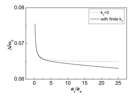
FIG. 2: Variation of mode splitting ( $\Delta = \omega_s - \omega_-$ ) with  $a_s/a_n$ . The other parameters are  $\omega_z = 2\pi \times 1000 Hz$ ,  $\omega_0 = 2\pi \times 20 Hz$ ,  $N = 10^4$ ,  $a_n = 27.5 A^0$  and  $\lambda = 0.8$ . The dotted curve shows  $\Delta$  values calculated within the mean-field theory (i.e.  $k_2 = 0$ ) whereas the continuous curve shows that with incorporating LHY term in the inteaction energy (i.e.  $k_2 = finite$ ).
