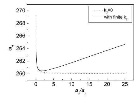
FIG. 1: Variation of monopole mode frequency with scattering length. The other parameters are  $N = 10^4$ ,  $\omega_z = 2\pi \times 1000 Hz$ ,  $\omega_0 = 2\pi \times 20 Hz$ ,  $a_n = 27.5 A^0$  and  $\lambda = 0.8$ . The dotted curve shows frequency values calculated within the mean-field theory (i.e.  $k_2 = 0$ ) whereas the continuous curve shows that after incorporating LHY correction term (i.e.  $k_2 = finite$ ).
