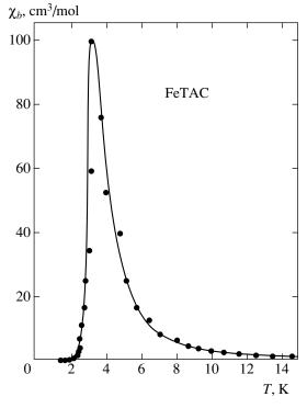
**Fig. 6.** Magnetic susceptibility of FeTAC along the crystallographic *b* axis: measurement data from [7] (symbols) and  $\chi_{\parallel}^{(10\times\infty)}(T)$  calculated for  $J/k_{\rm B} = 16.6$  K,  $g_{\parallel} = 7.67$ , and  $J/J = -1.38 \times 10^{-3}$  (curve).
