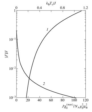
**Fig. 5.** Reduced critical temperature (curve *1*) and maximum value of normalized longitudinal susceptibility (curve 2) vs. |J'|/J for 2D superantiferromagnetic Ising lattices.
