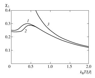
**Fig. 2.** Zero-field transverse susceptibility (measured in units of  $N_A g_{\perp}^2 \mu_B^2 / J$ ) vs. normalized temperature: (1) 1D chain (J' = 0); (2) double chain with z' |J' / J| = 0.1; (3) free spins (J = J' = 0).
