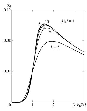
**Fig. 3.** Longitudinal susceptibility for  $L \times \infty$  superantiferromagnetic Ising strips with L = 2-10 and |J'|/J = 1 (measured in units of  $N_A g_{\parallel}^2 \mu_B^2 / J$ ).
