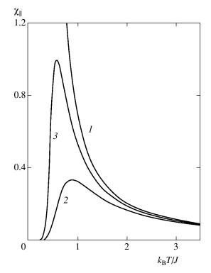
**Fig. 1.** Longitudinal susceptibility for Ising chain models (measured in units of  $N_A g_{\parallel}^2 \mu_B^2 / J$ ) vs. normalized temperature: (1) linear ferromagnetic chain; (2) double chain with z'J'/J = -0.5 (J > 0); (3) four-chain cylinder with J > 0 and z'J'/2J = -0.1.
