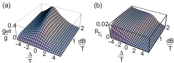
FIG. 2: (a) Coupling strength,  $g_{\text{eff}}$ , in units of bare coupling  $g$ , as a function of field gradient  $dB$  and bias  $\Delta_0$ . (b) Calculated probability of error in swapping a double-dot state with the resonator state due to charge-based relaxation using  $t = 4 \mu\text{eV}$  and an inverse temperature of  $10 \mu\text{eV}$ .
